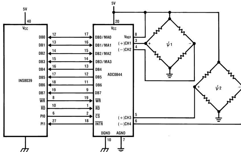
Figure 23. ADC0844—INS8039 Interface
