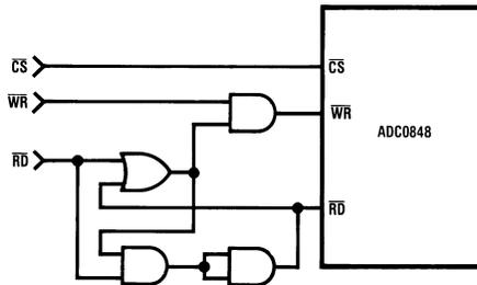
$\overline{CS} \cdot \overline{WR}$  will update the channel configuration and start a conversion.
