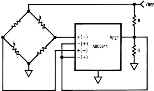
Figure 16. Differential Voltage Input 9-Bit A/D
