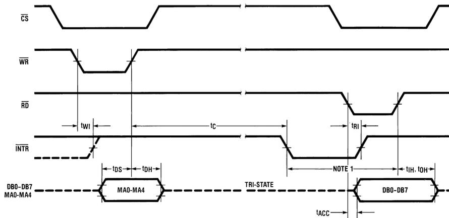
Read strobe must occur at least 600 ns after the assertion of interrupt to ensure reset of  $\overline{\text{INTR}}$ .
