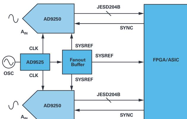
Figure 1. Diagram showing the AD9250, the AD9525, and an FPGA.
