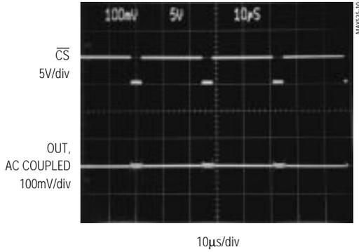
DIGITAL FEEDTHROUGH ( $f_{SCLK} = 100kHz$ )
