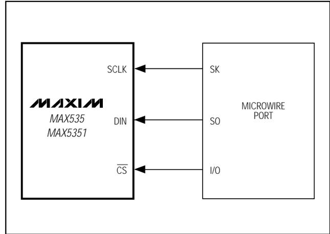
Figure 2. Connections for Microwire
