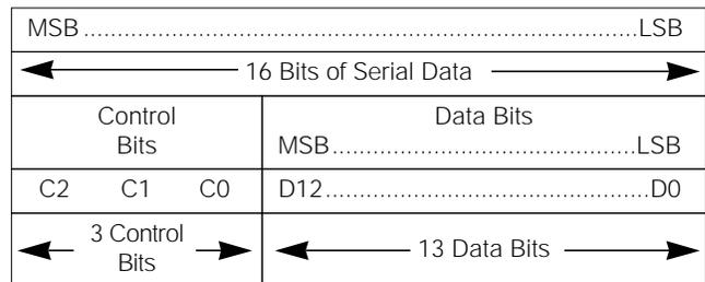
Figure 4. Serial-Data Format
