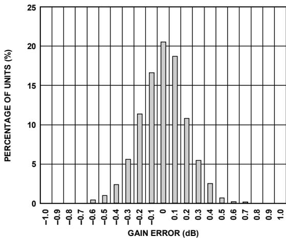
Figure 10. Gain Error Histogram,  $V_{GAIN} = -1.28$  V
