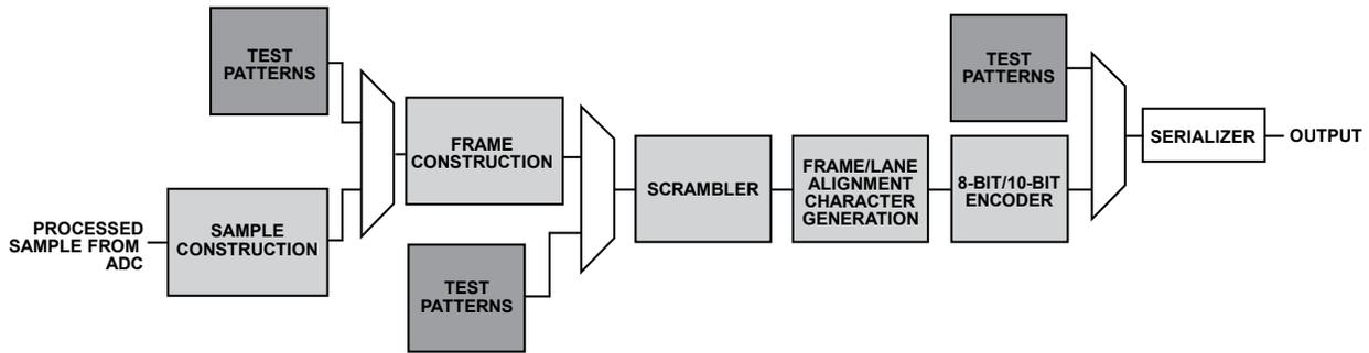
Figure 55. Example of Data Flow Block Diagram
