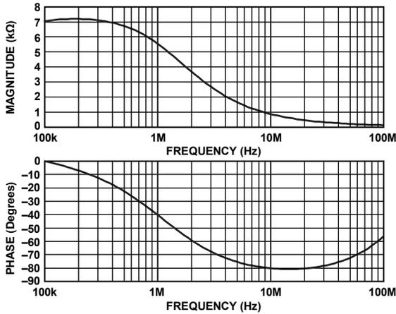
Figure 27. LNA Input Impedance Magnitude and Phase, Unterminated
