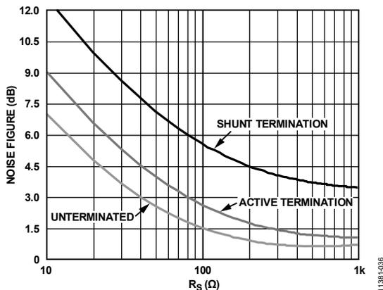
Figure 35. Noise Figure vs. R<sub>S</sub> for Shunt Termination, Active Termination Matched and Unterminated Inputs, V<sub>GAIN</sub> = 1.6 V
