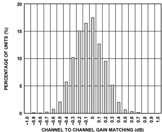
Figure 14. Gain Matching Histogram,  $V_{GAIN} = 1.2$  V
