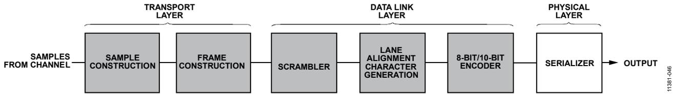
Figure 45. AD9675 Transmit Link Simplified Block Diagram
