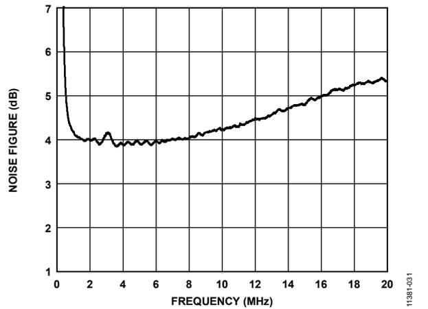
Figure 30. Noise Figure vs. Frequency
