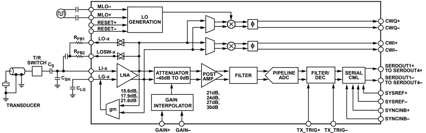
Figure 33. Simplified Block Diagram of a Single Channel
