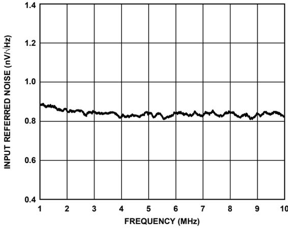
Figure 15. Short-Circuit, Input Referred Noise vs. Frequency
