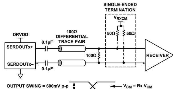
Figure 47. AC-Coupled Digital Output Termination Example
