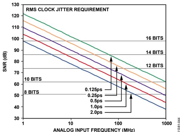
Figure 43. Ideal SNR vs. Input Frequency and Jitter
