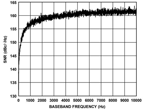
Figure 32. Output Referred SNR vs. Baseband Frequency
