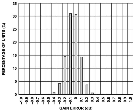
Figure 11. Gain Error Histogram,  $V_{GAIN} = 0$  V
