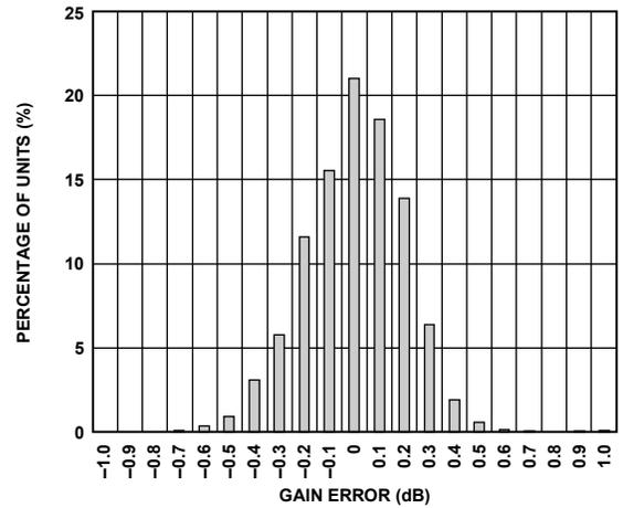
Figure 12. Gain Error Histogram,  $V_{GAIN} = 1.28$  V
