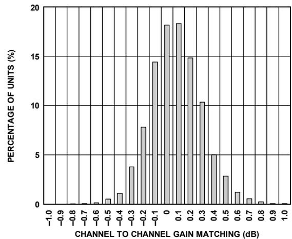
Figure 13. Gain Matching Histogram,  $V_{GAIN} = -1.2$  V
