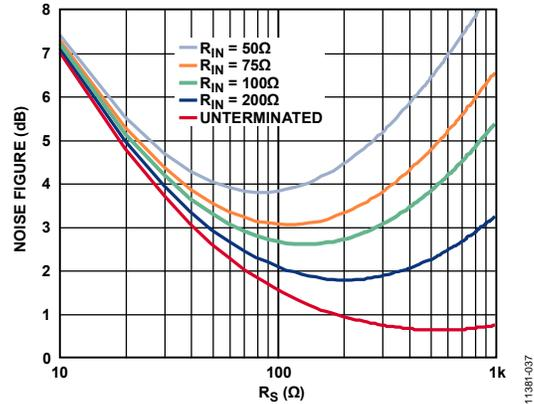
Figure 36. Noise Figure vs. R<sub>S</sub> for Various Fixed Values of R<sub>IN</sub>, Active Termination Matched Inputs, V<sub>GAIN</sub> = 1.6 V
