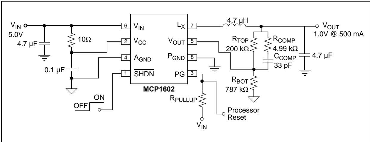
**FIGURE 6-2:** 5V to 1.0V @ 500 mA Application.
