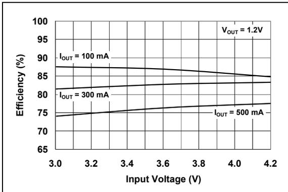
**FIGURE 2-2:** Efficiency vs. Input Voltage ( $V_{OUT} = 1.2V$ ).
