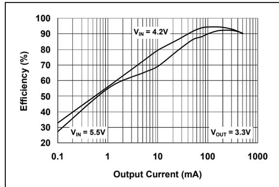
**FIGURE 2-10:** Efficiency vs. Output Load ( $V_{OUT} = 3.3\text{V}$ ).
