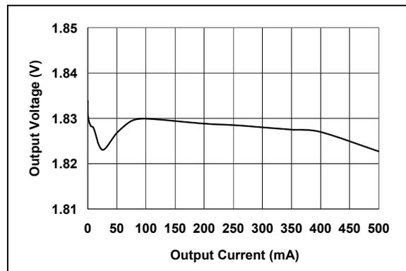
**FIGURE 2-12:** Output Voltage vs. Load Current ( $V_{OUT} = 1.8\text{V}$ ).
