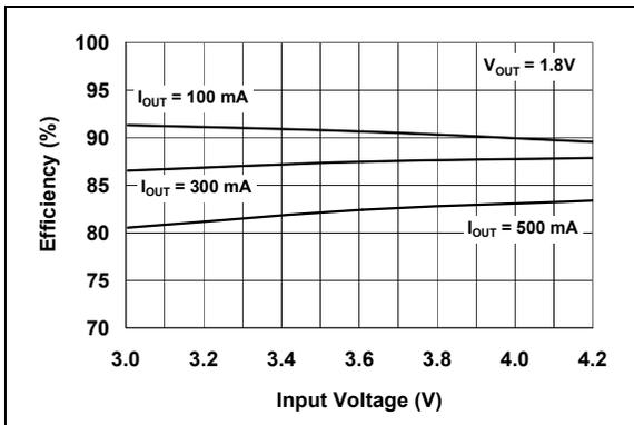
**FIGURE 2-3:** Efficiency vs. Input Voltage ( $V_{OUT} = 1.8V$ ).
