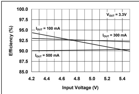
**FIGURE 2-7:** Efficiency vs. Input Voltage ( $V_{OUT} = 3.3\text{V}$ ).
