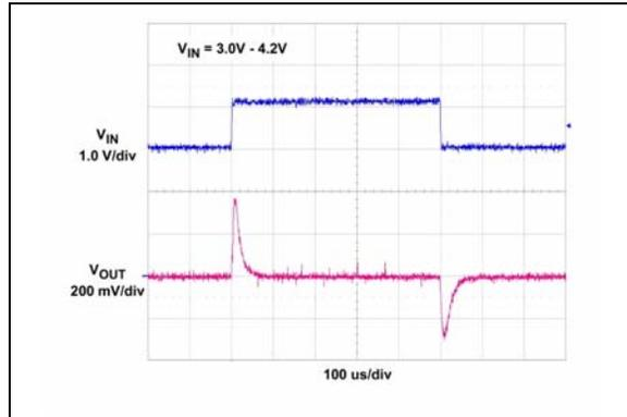
**FIGURE 2-21:** Output Voltage Line Step Response vs. Time.
