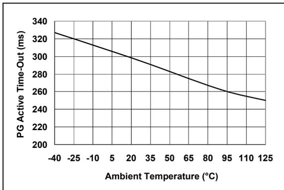
**FIGURE 2-8:** PG Active Time-out vs. Ambient Temperature.
