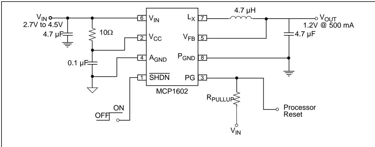
**FIGURE 6-3:** 3 NiMH Batteries to 1.2V @ 500 mA Application.
