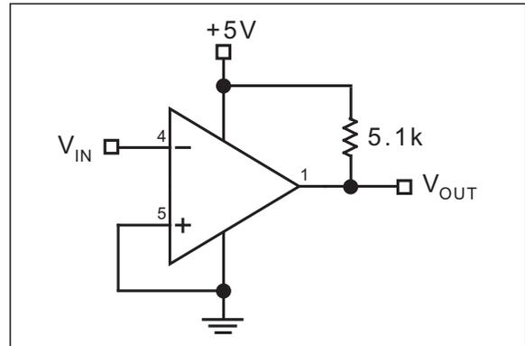
**FIGURE 2-4:** Output Response Time vs. Overdrive (Test Circuit).
