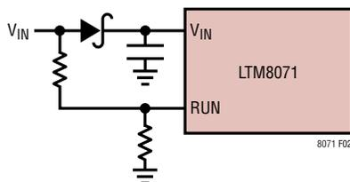
**Figure 2. The Input Diode Prevents a Shorted Input from Discharging a Backup Battery Tied to the Output. It Also Protects the Circuit from a Reversed Input. The LTM8071 Runs Only When the Input Is Present.**
