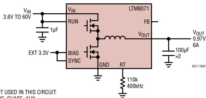
PINS NOT USED IN THIS CIRCUIT:
