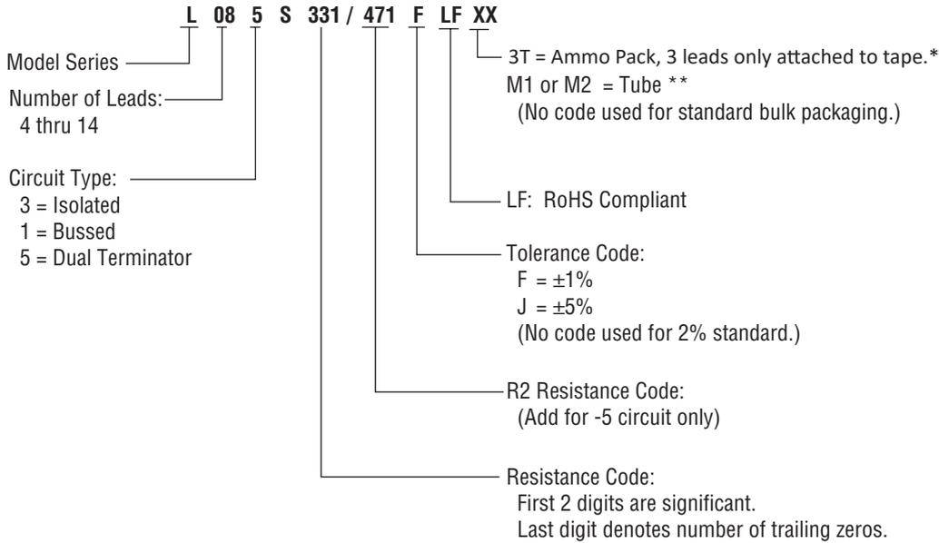
\* Refer to Packaging for Automation section (Page A-3) for Ammo Pack capacity and dimensions.
