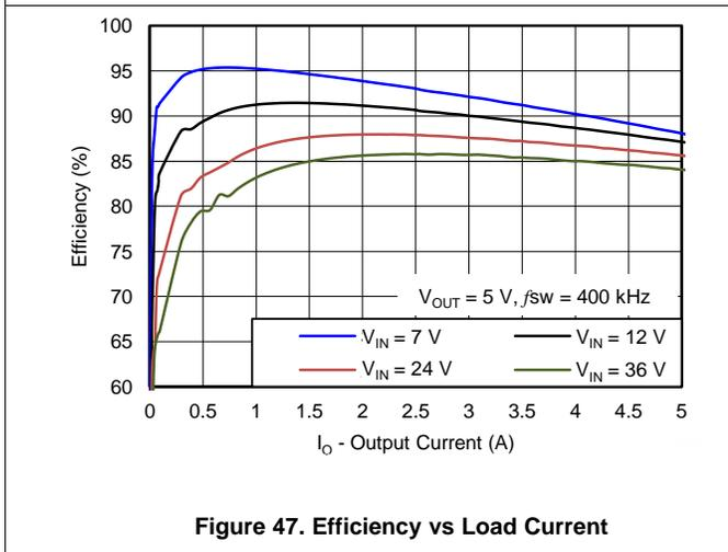
Figure 47. Efficiency vs Load Current
