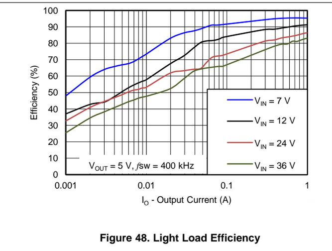
Figure 48. Light Load Efficiency
