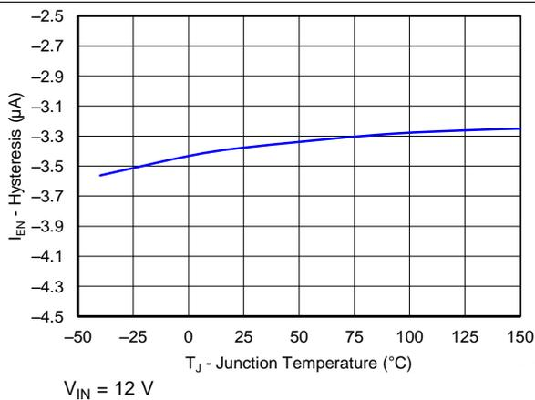
Figure 13. EN Pin Current Hysteresis vs Junction Temperature
