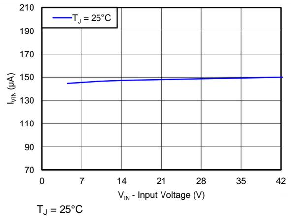
Figure 18.  $V_{IN}$  Supply Current vs Input Voltage
