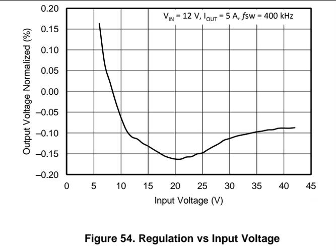
**Figure 54. Regulation vs Input Voltage**
