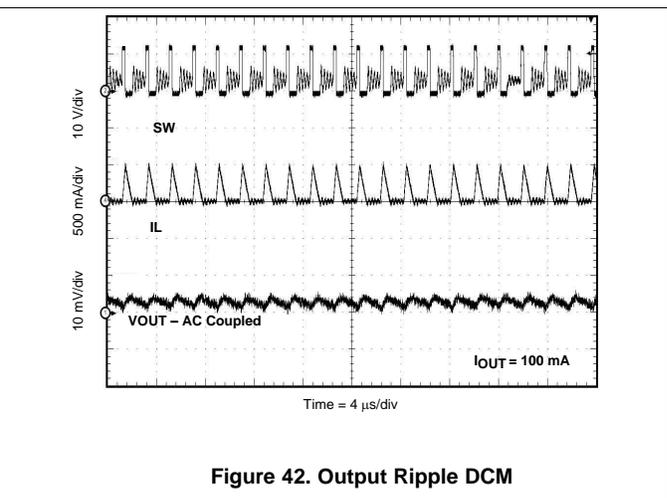
Measurements are taken with standard EVM using a 12-V input, 3.3-V output, and 5-A load unless otherwise noted.
