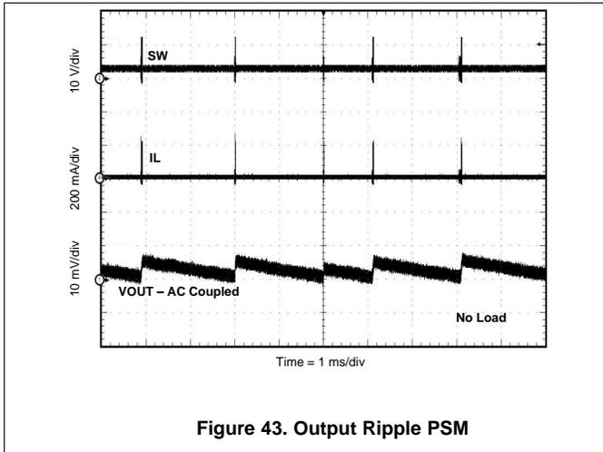
Figure 43. Output Ripple PSM
