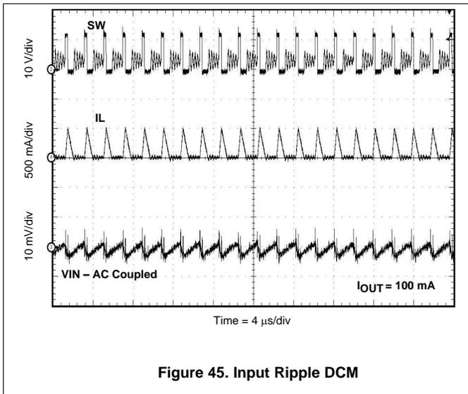
Figure 45. Input Ripple DCM
