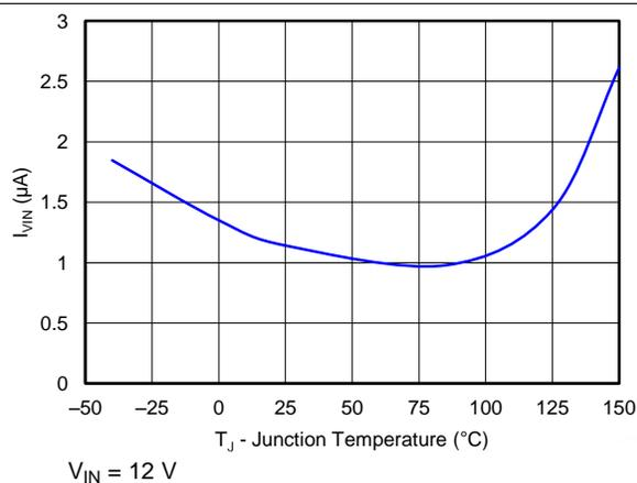
Figure 15. Shutdown Supply Current vs Junction Temperature
