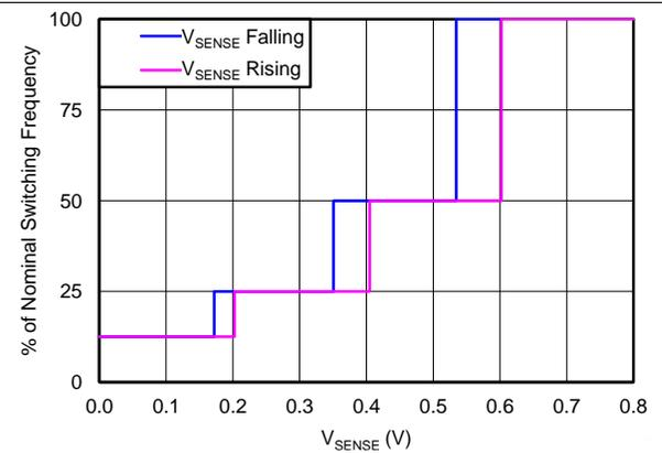
Figure 14. Switching Frequency vs V<sub>SENSE</sub>
