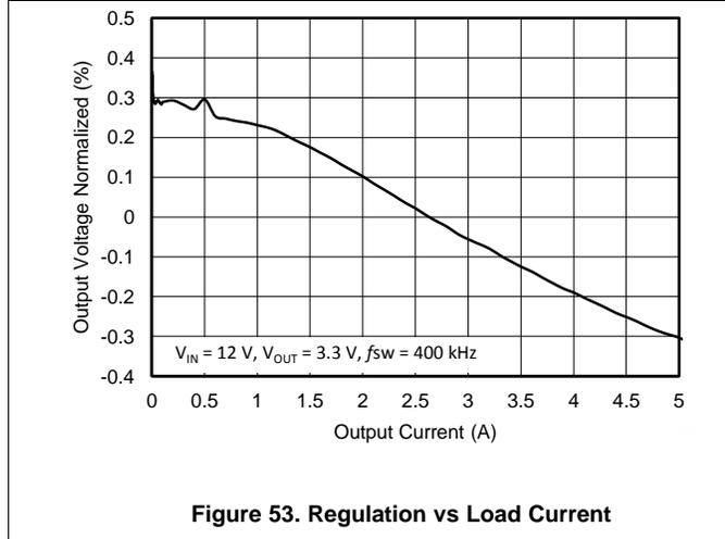
**Figure 53. Regulation vs Load Current**
