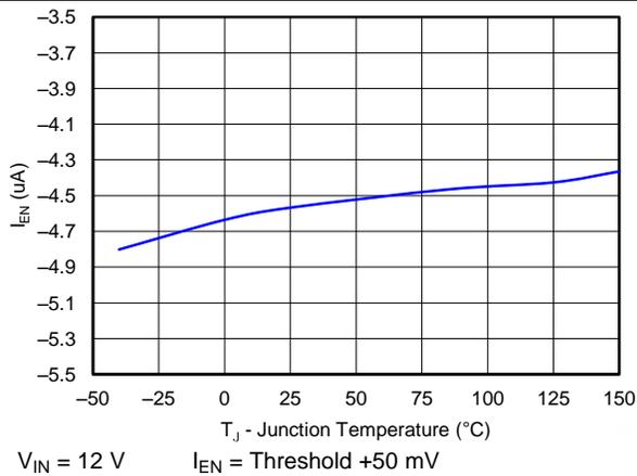
Figure 11. EN Pin Current vs Junction Temperature
