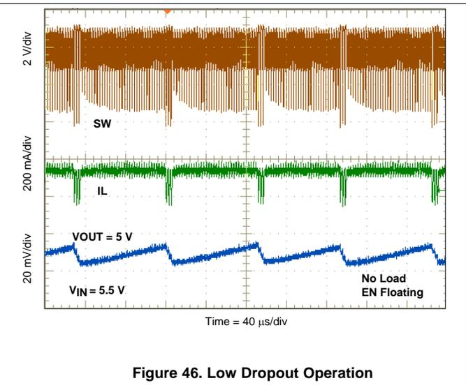
Figure 46. Low Dropout Operation
