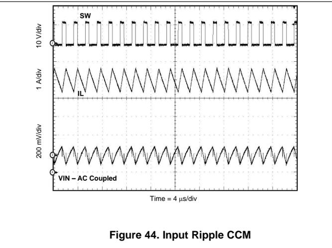
Figure 44. Input Ripple CCM
