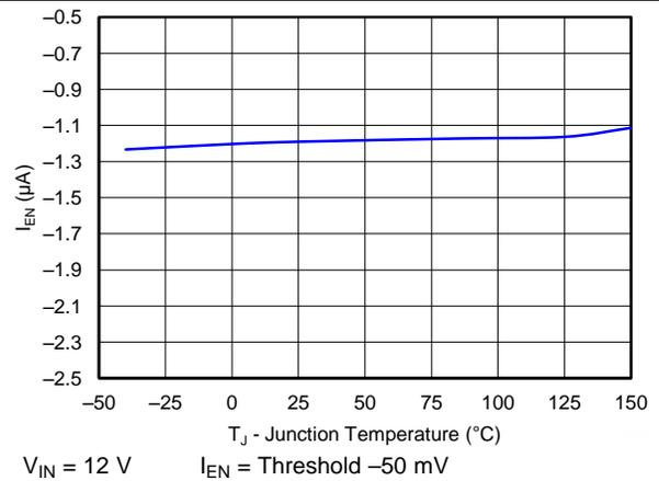
Figure 12. EN Pin Current vs Junction Temperature
