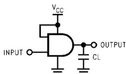
C<sub>L</sub> includes load and stray capacitance
