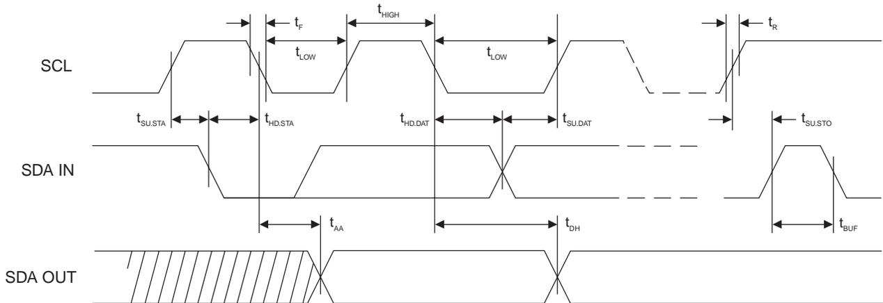
**Figure 5-2. Write Cycle Timing**
