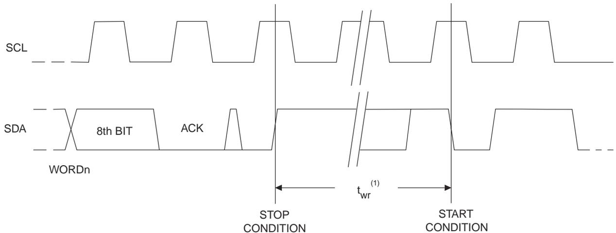
Note: The write cycle time  $t_{wr}$  is the time from a valid stop condition of a write sequence to the end of the internal clear/write cycle
