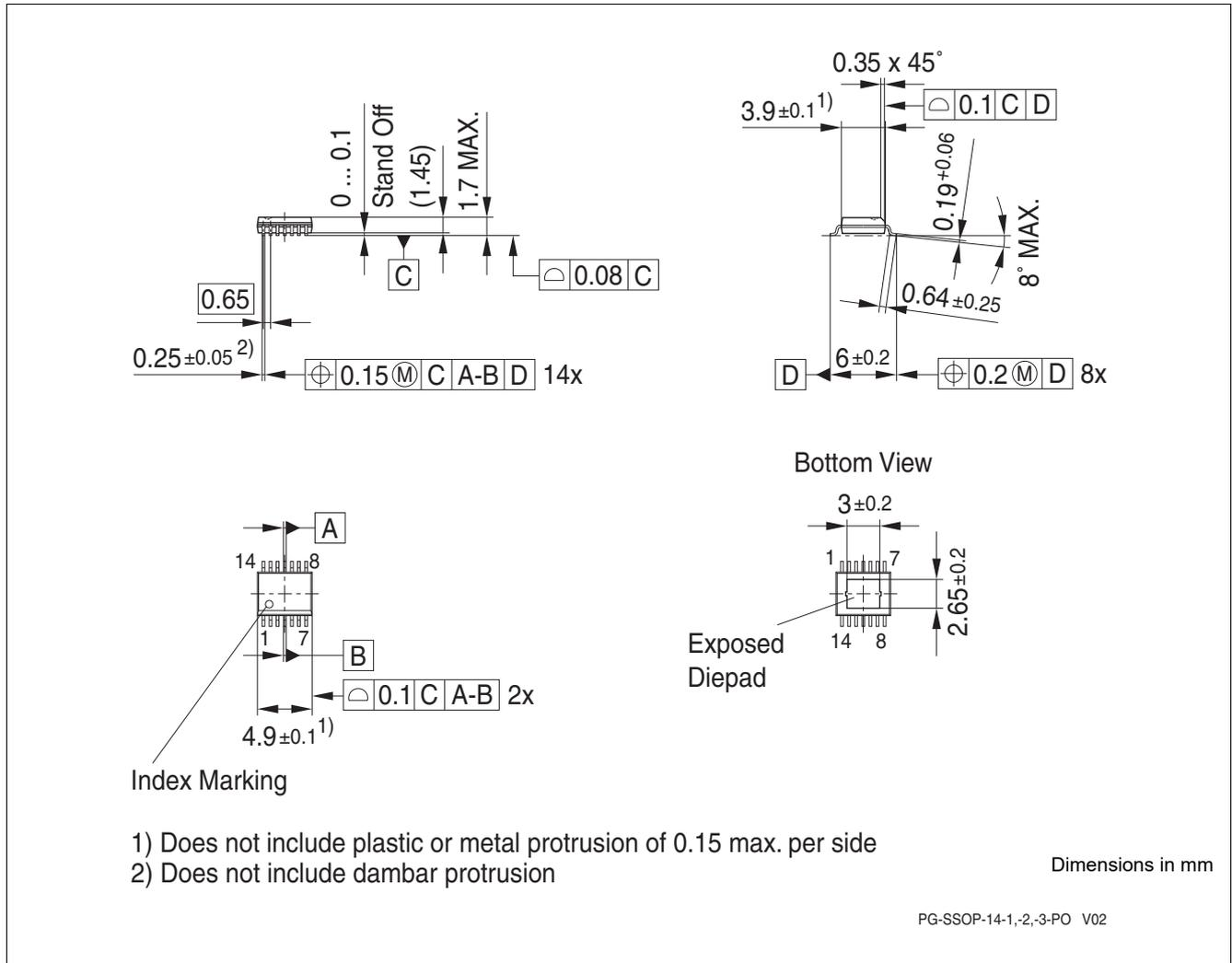
**Figure 21 PG-SSOP-14**
