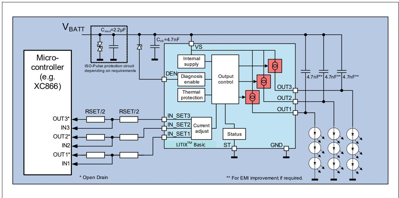
Figure 20 Application Diagram with Diagnosis for each channel
