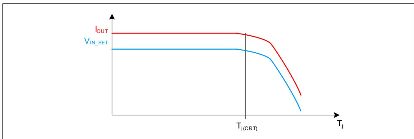
**Figure 19 Output current reduction at high temperature**
