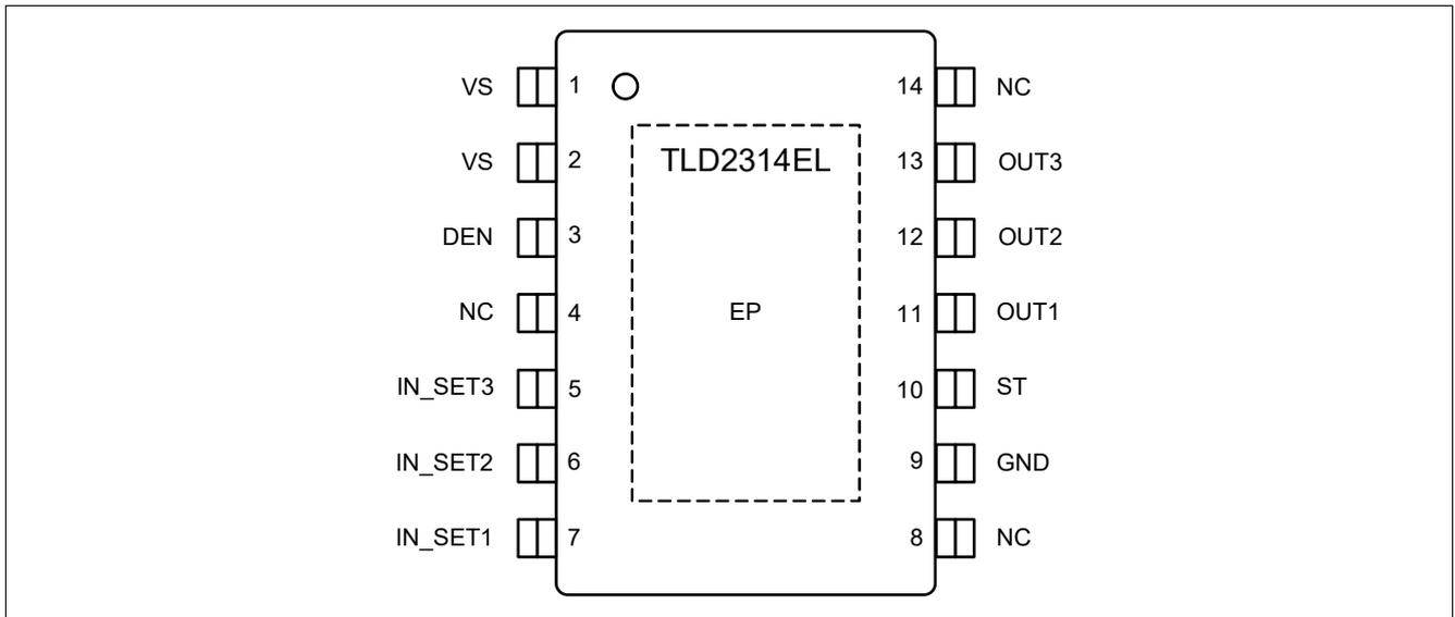
Figure 2 Pin Configuration
