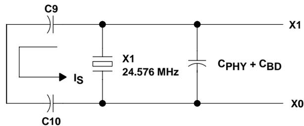
**Figure 8–4. Load Capacitance for the TSB43AB23 PHY**
