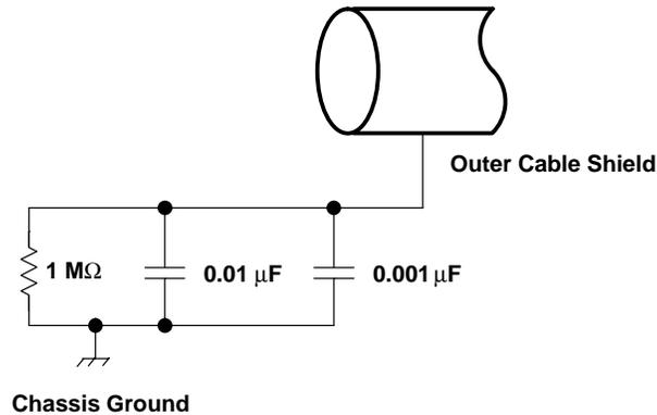
**Figure 8–2. Typical Compliant DC Isolated Outer Shield Termination**
