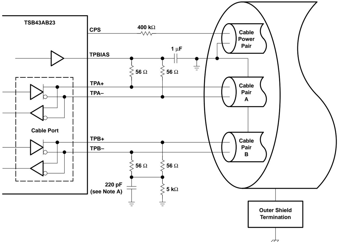
NOTE A: IEEE Std 1394-1995 calls for a 250-pF capacitor, which is a nonstandard component value. A 220-pF capacitor is recommended.
