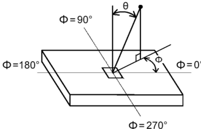
6. 3D performance specification is expressed by 3D luminance, 3D Crosstalk and 3D viewing angle. 3D luminance which is defined by summation of left and right eye brightness under wearing glasses condition is measured at panel center point. Also, 3D crosstalk is measured at panel center point.
