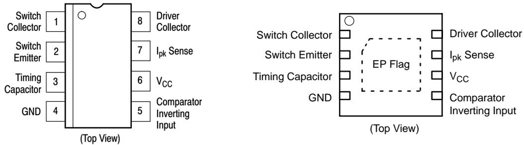
Figure 2. Pin Connections
