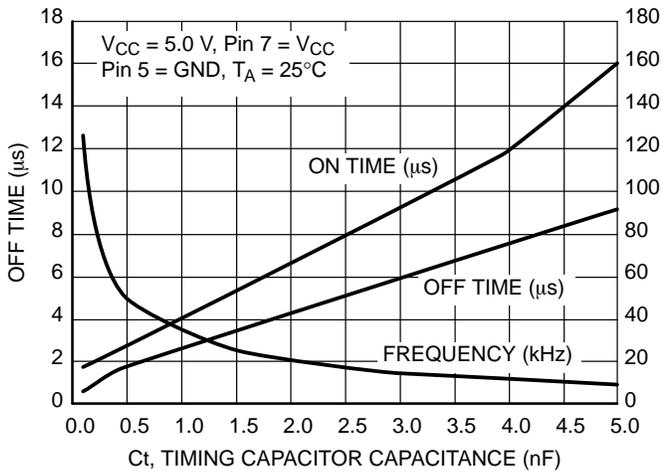
Figure 3. Oscillator Frequency
