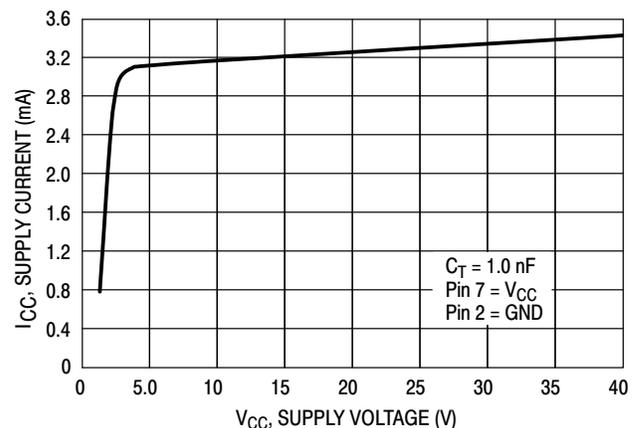
Figure 8. Standby Supply Current versus Supply Voltage
