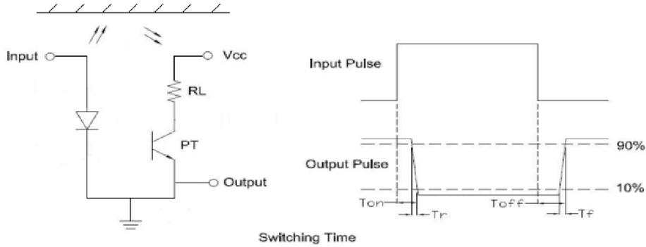
Light Current Measurement Setup Diagram :
