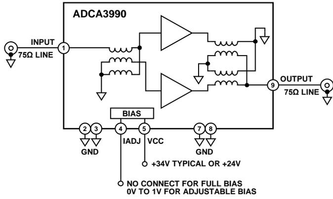
Figure 10. Basic Connections
