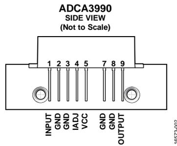
Figure 2. Pin Configuration
