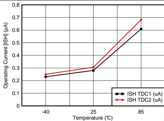
Figure 19. Shutdown Current (ISH) vs Temperature
