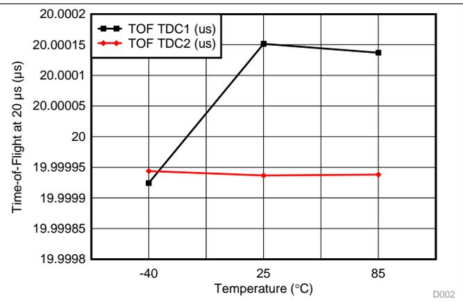
Figure 3. TOF vs Temperature (Measurement Mode 2)
