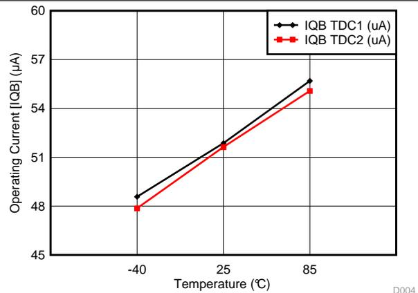
Figure 13. Operating Current (IQB) vs Temperature
