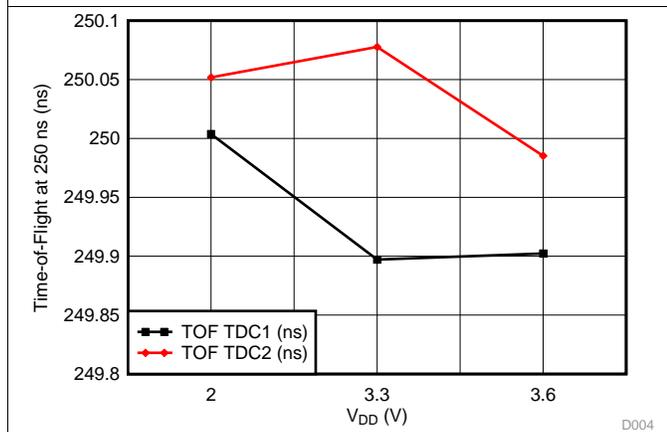
Figure 4. TOF vs VDD (Measurement Mode 1)
