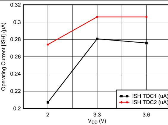
Figure 18. Shutdown Current (ISH) vs VDD
