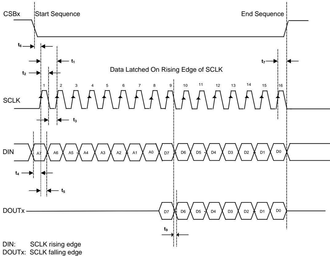
**Figure 1. SPI Register Access: 8 Bit Register Example**
