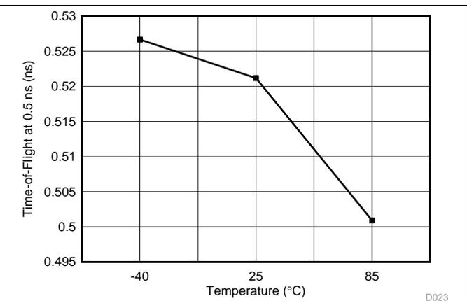
Figure 7. TOF vs. Temperature (Mode 1 Combined Operation)
