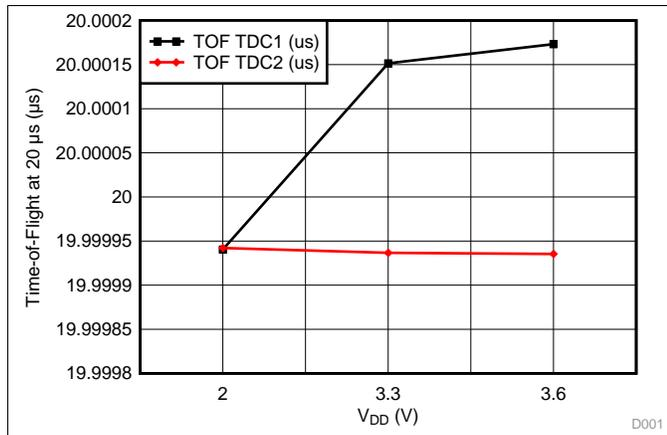
Figure 2. Time-of-Flight (TOF) vs VDD (Measurement Mode 2)
