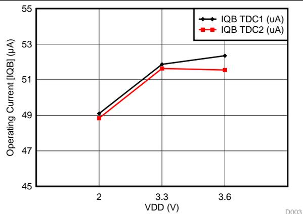
Figure 12. Operating Current (IQB) vs VDD
