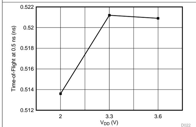
Figure 6. TOF vs. VDD (Mode 1 Combined Operation)
