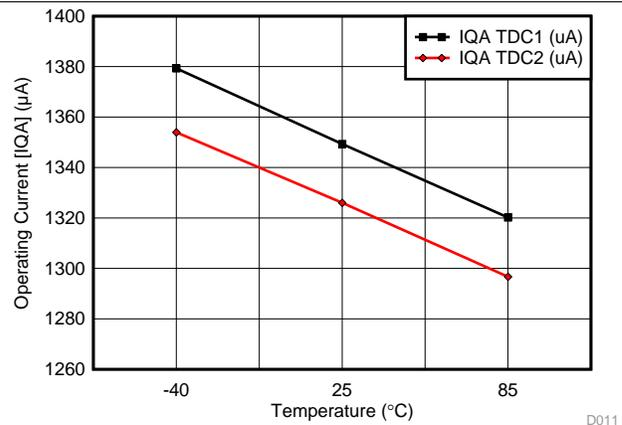
Figure 11. Operating Current (IQA) vs Temperature
