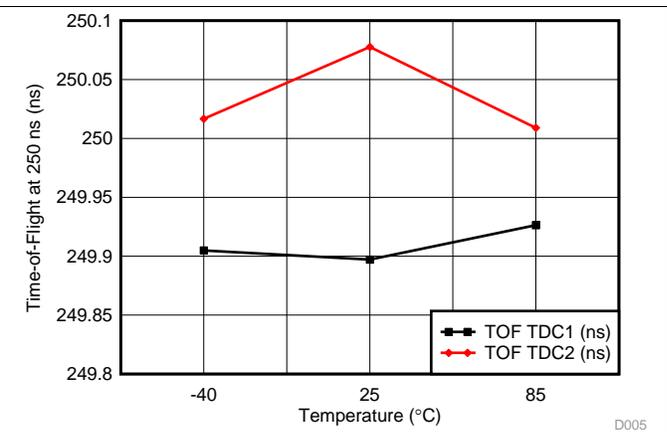
Figure 5. TOF vs Temperature (Measurement Mode 1)
