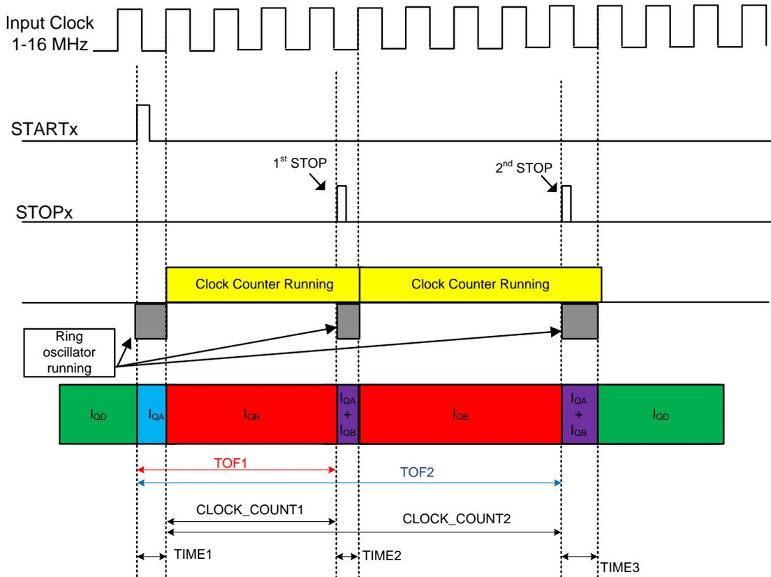
Figure 23. Measurement Mode 2
