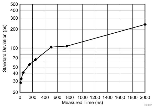
**Figure 22. Measurement Mode 1 Standard Deviation vs Measured Time-of-Flight**
