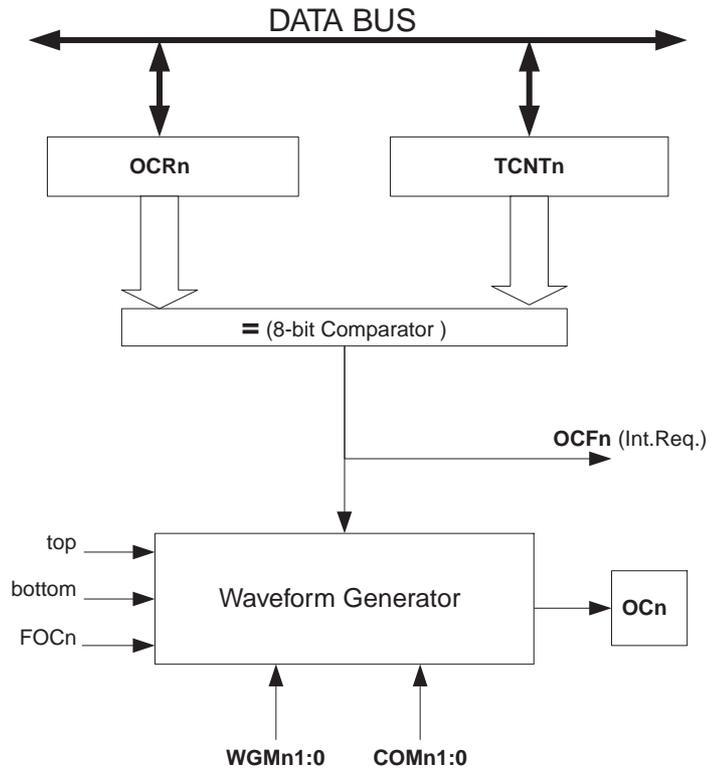
The OCR0 Register is double buffered when using any of the Pulse Width Modulation (PWM) modes. For the Normal and Clear Timer on Compare (CTC) modes of operation, the double buffering is disabled. The double buffering synchronizes the update of the OCR0 Compare Register to either top or bottom of the counting sequence. The synchronization prevents the occurrence of odd-length, non-symmetrical PWM pulses, thereby making the output glitch-free.
