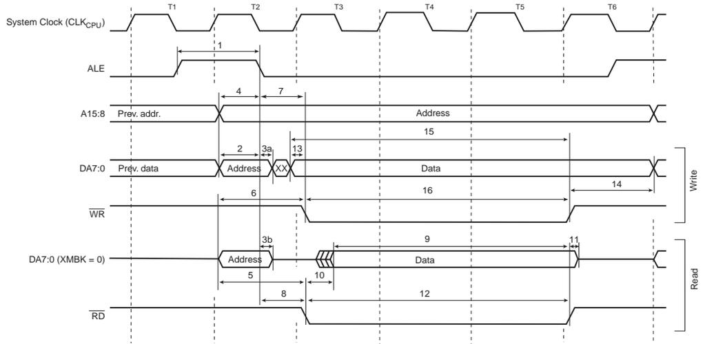
**Figure 119. External Memory Timing (SRWn1 = 1, SRWn0 = 1)<sup>(1)</sup>**
