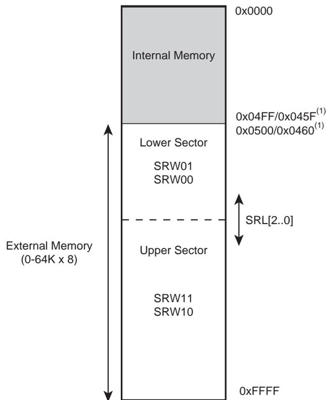
Note: 1. Address depends on the ATmega161 compability Fuse. See “SRAM Data Memory” on page 16 and Figure 9 on page 17 for details.
