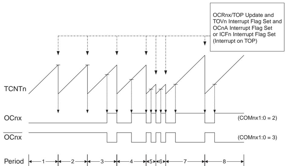
The Timer/Counter Overflow Flag (TOVn) is set each time the counter reaches TOP. In addition the OCnA or ICFn flag is set at the same timer clock cycle as TOVn is set when
