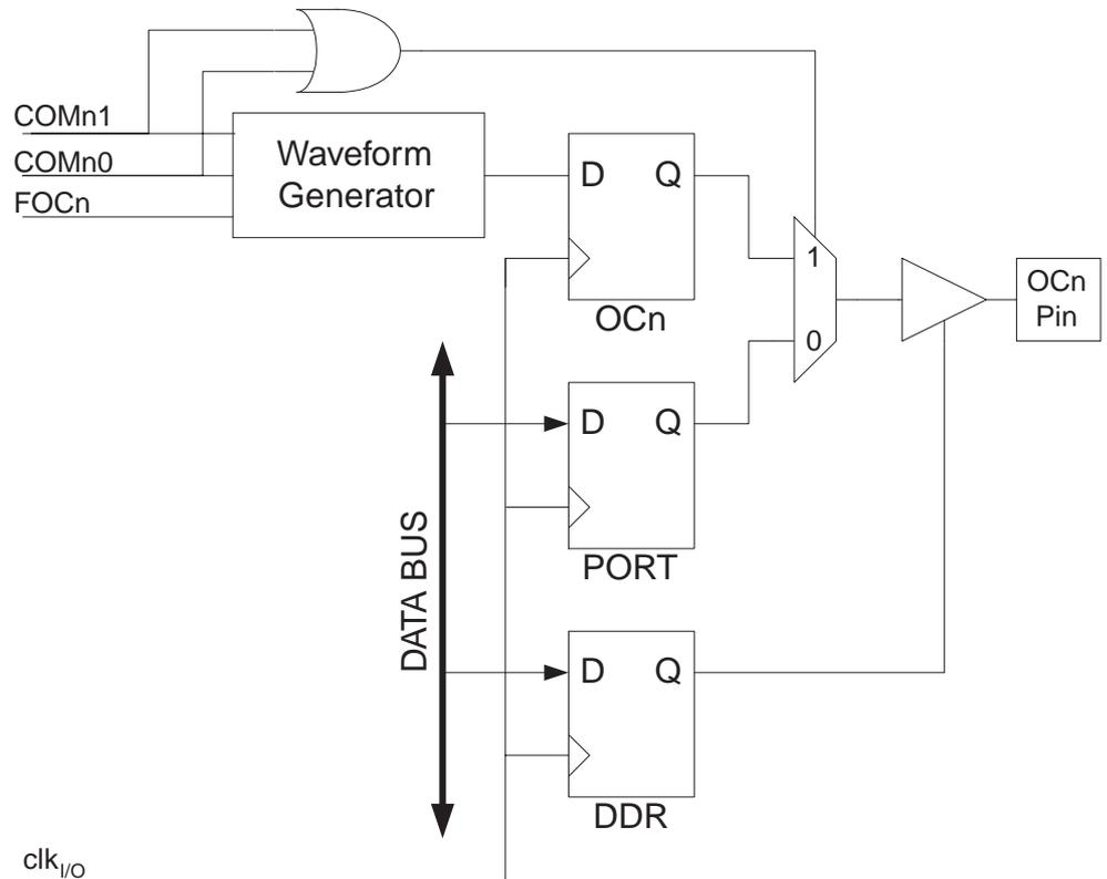
The general I/O port function is overridden by the Output Compare (OC2) from the waveform generator if either of the COM21:0 bits are set. However, the OC2 pin direction (input or output) is still controlled by the Data Direction Register (DDR) for the port pin. The Data Direction Register bit for the OC2 pin (DDR\_OC2) must be set as output before the OC2 value is visible on the pin. The port override function is independent of the Waveform Generation mode.
