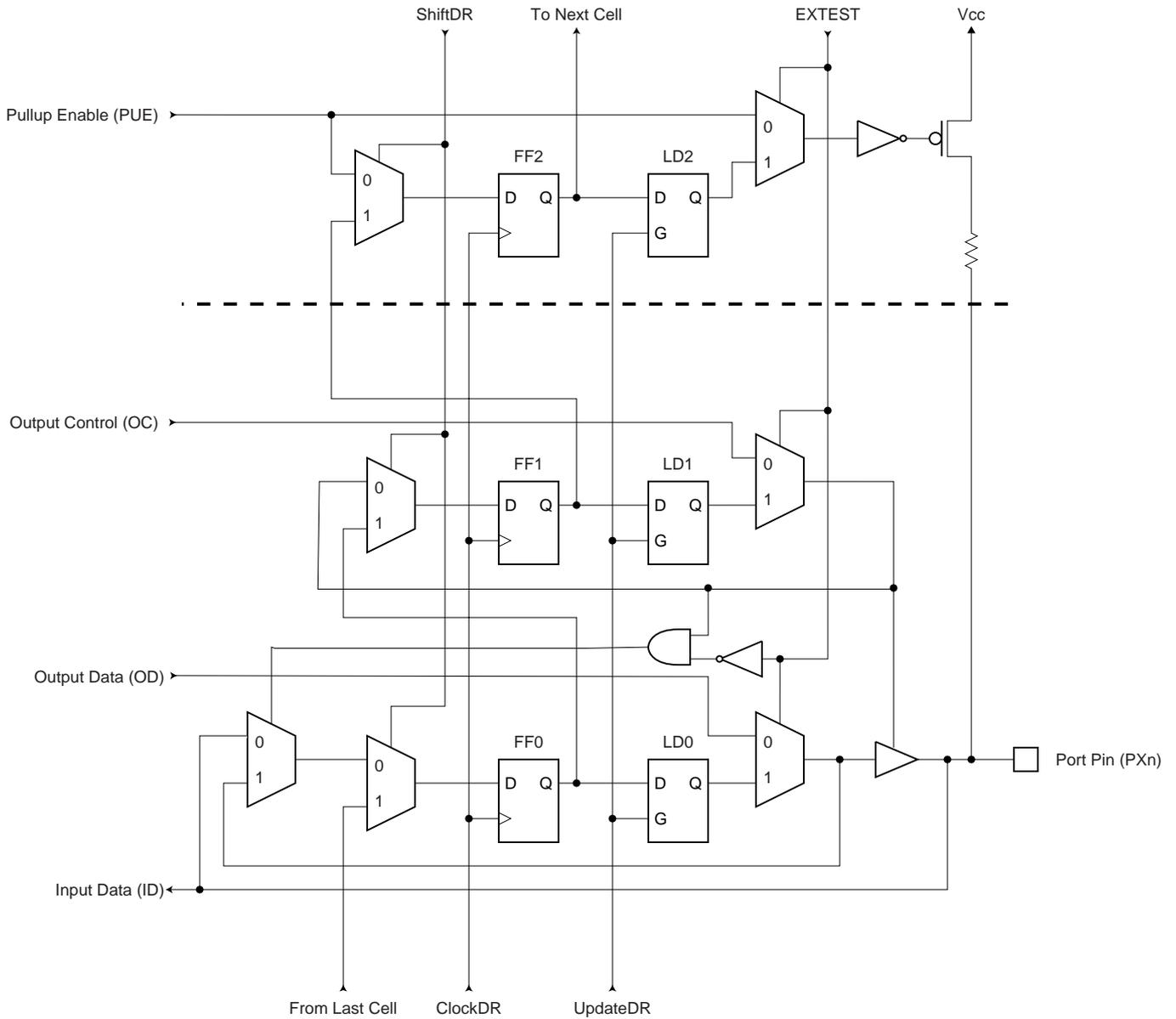
**Figure 88. General Port Pin Schematic Diagram**
