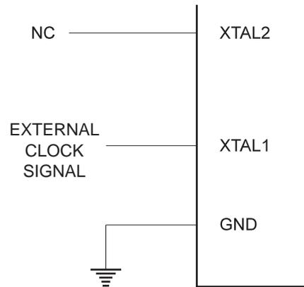
When this clock source is selected, start-up times are determined by the SUT Fuses as shown in Table 14.
