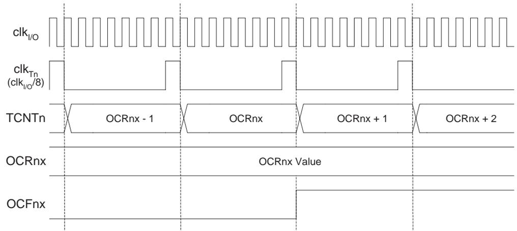
Figure 57 shows the count sequence close to TOP in various modes. When using phase and frequency correct PWM mode the OCRnx Register is updated at BOTTOM. The timing diagrams will be the same, but TOP should be replaced by BOTTOM, TOP-1 by BOTTOM+1 and so on. The same renaming applies for modes that set the TOVn flag at BOTTOM.
