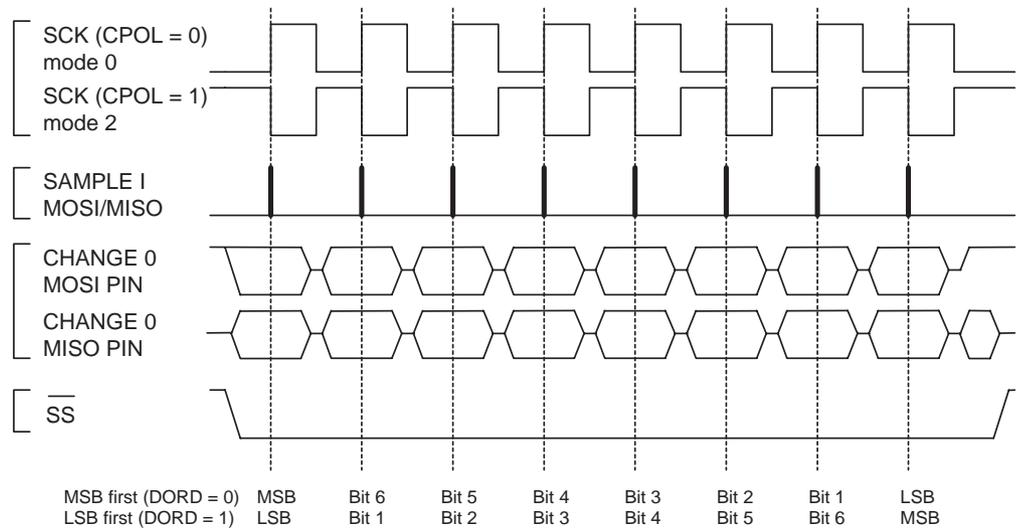
**Figure 74.** SPI Transfer Format with CPHA = 1
