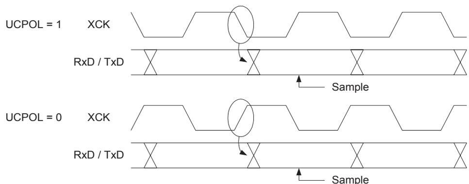
The UCPOL bit UCRSC selects which XCK clock edge is used for data sampling and which is used for data change. As Figure 77 shows, when UCPOL is zero the data will be changed at rising XCK edge and sampled at falling XCK edge. If UCPOL is set, the data will be changed at falling XCK edge and sampled at rising XCK edge.
