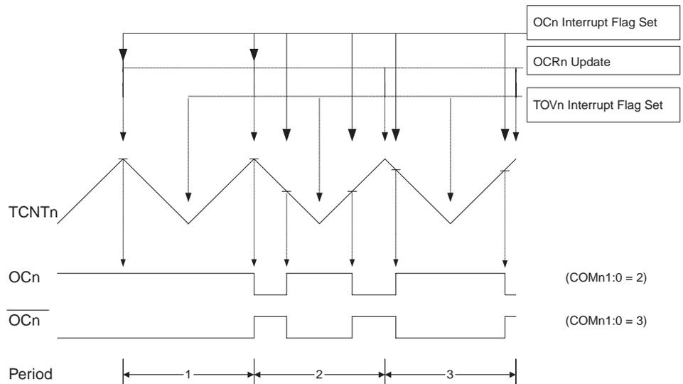
The Timer/Counter Overflow Flag (TOV2) is set each time the counter reaches BOTTOM. The interrupt flag can be used to generate an interrupt each time the counter reaches the BOTTOM value.
