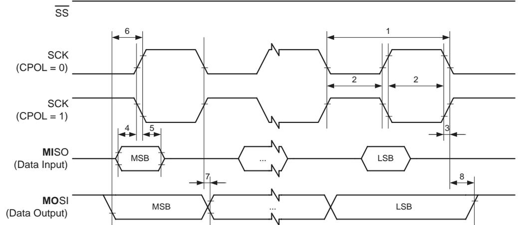
**Figure 115. SPI Interface Timing Requirements (Slave Mode)**
