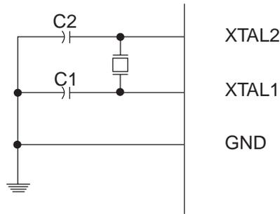
The Oscillator can operate in four different modes, each optimized for a specific frequency range. The operating mode is selected by the fuses CKSEL3:1 as shown in Table 7.
