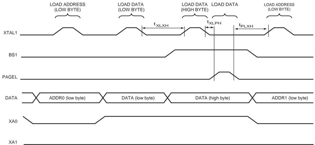
Note: 1. The timing requirements shown in Figure 102 (i.e.,  $t_{DVXH}$ ,  $t_{XHL}$ , and  $t_{XLDX}$ ) also apply to loading operation.
