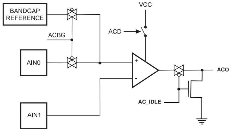
**Figure 92.** General Boundary-scan Cell used for Signals for Comparator and ADC
