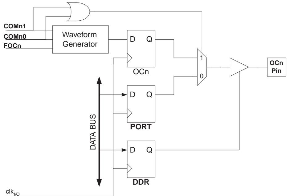
The general I/O port function is overridden by the Output Compare (OC0) from the waveform generator if either of the COM01:0 bits are set. However, the OC0 pin direction (input or output) is still controlled by the Data Direction Register (DDR) for the port pin. The Data Direction Register bit for the OC0 pin (DDR\_OC0) must be set as output before the OC0 value is visible on the pin. The port override function is independent of the Waveform Generation mode.
