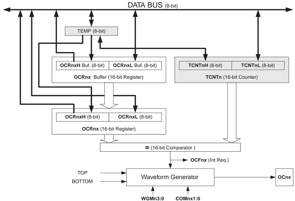
The OCRnx Register is double buffered when using any of the twelve *Pulse Width Modulation* (PWM) modes. For the normal and *Clear Timer on Compare* (CTC) modes of operation, the double buffering is disabled. The double buffering synchronizes the update of the OCRnx Compare Register to either TOP or BOTTOM of the counting
