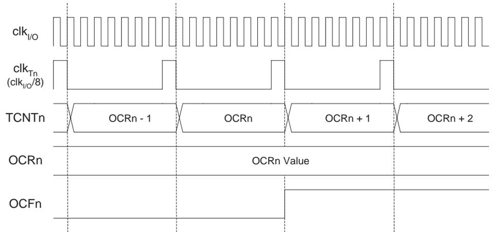
Figure 69 shows the setting of OCF2 and the clearing of TCNT2 in CTC mode.
