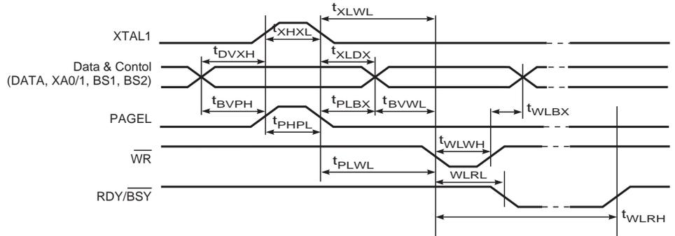
**Figure 103.** Parallel Programming Timing, Loading Sequence with Timing Requirements<sup>(1)</sup>
