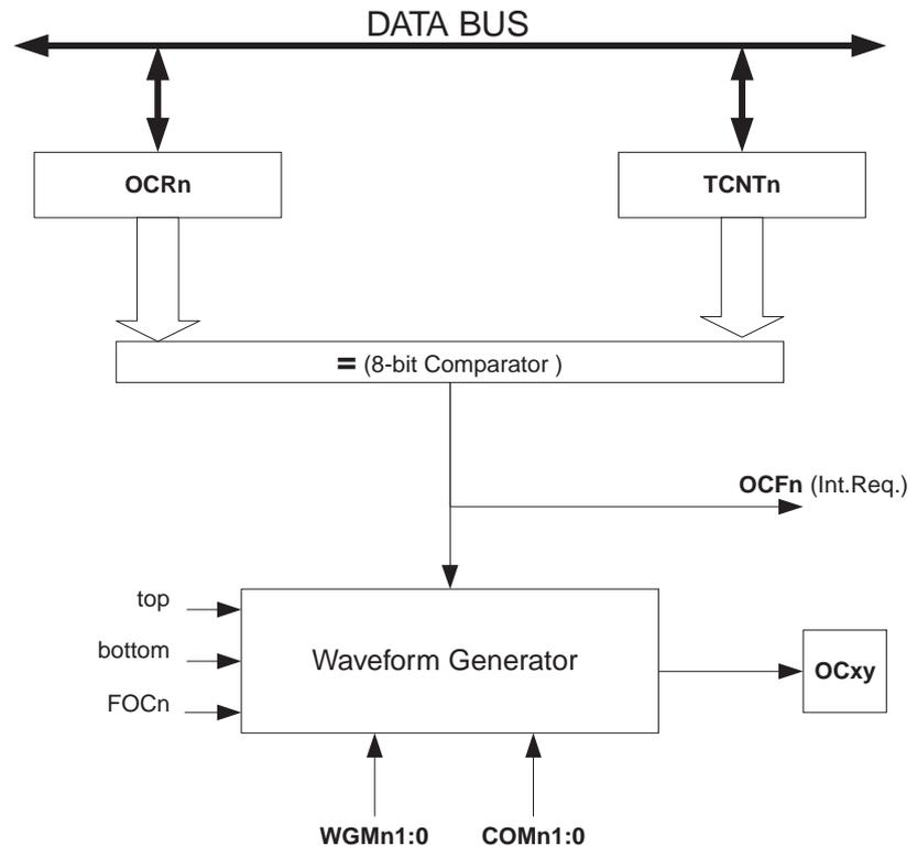
The OCR2 Register is double buffered when using any of the Pulse Width Modulation (PWM) modes. For the normal and Clear Timer on Compare (CTC) modes of operation, the double buffering is disabled. The double buffering synchronizes the update of the OCR2 Compare Register to either top or bottom of the counting sequence. The synchronization prevents the occurrence of odd-length, non-symmetrical PWM pulses, thereby making the output glitch-free.
