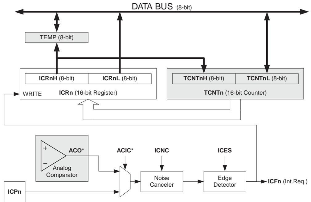
Note: 1. The Analog Comparator Output (ACO) can only trigger the Timer/Counter1 ICP – not Timer/Counter3.
