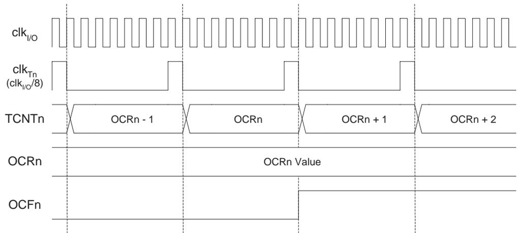
Figure 43 shows the setting of OCF0 and the clearing of TCNT0 in CTC mode.
