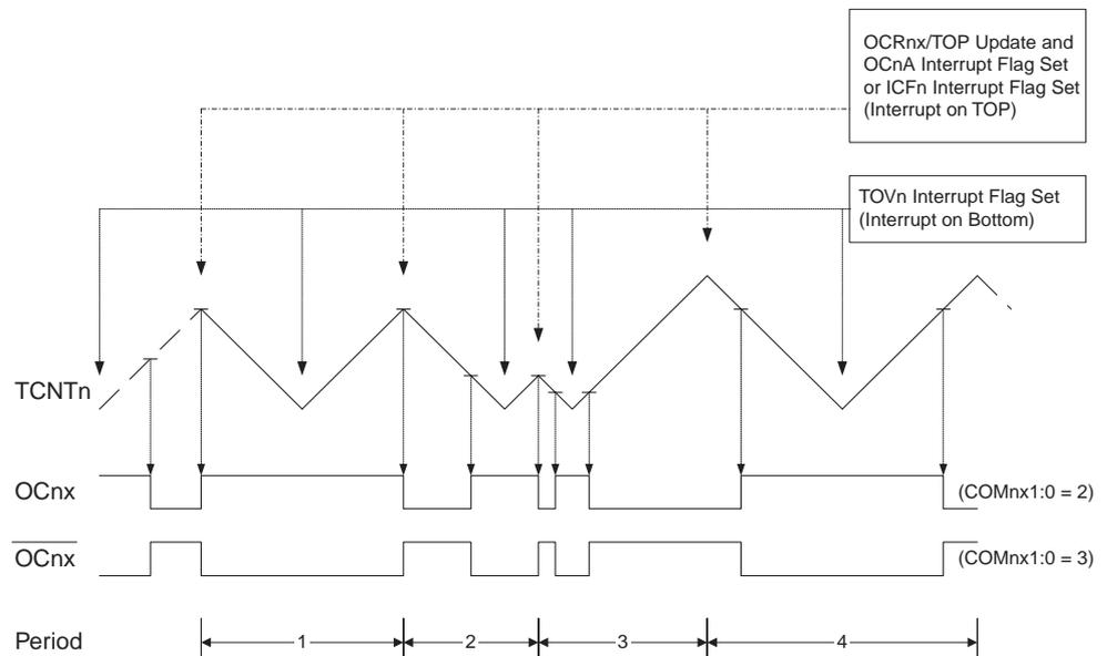
The Timer/Counter Overflow Flag (TOVn) is set each time the counter reaches BOTTOM. When either OCRnA or ICRn is used for defining the TOP value, the OCnA or
