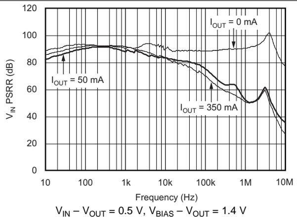
Figure 18.  $V_{IN}$  Power-Supply Rejection Ratio vs Frequency
