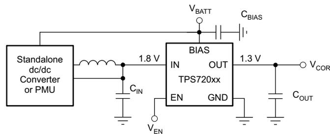
Figure 26. Typical Application Schematic
