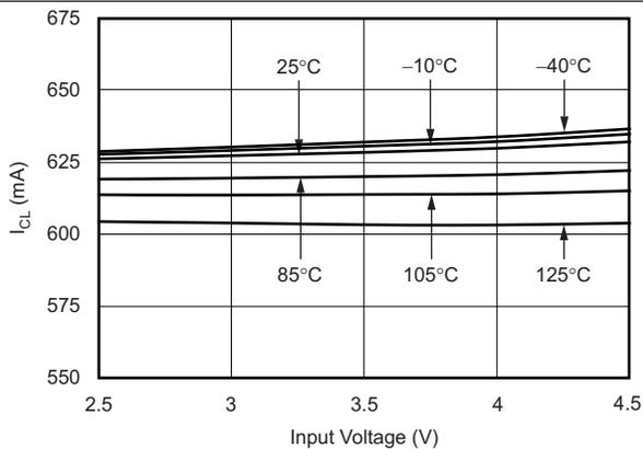
Figure 17. Current Limit vs Input Voltage
