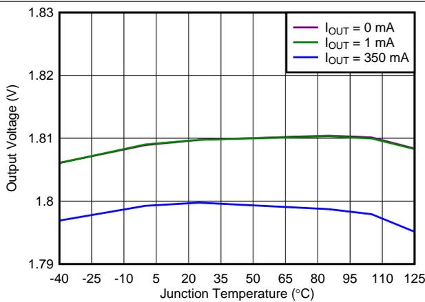
Figure 11. Output Voltage vs Junction Temperature
