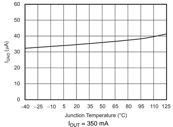
Figure 14. Ground Pin Current vs Junction Temperature
