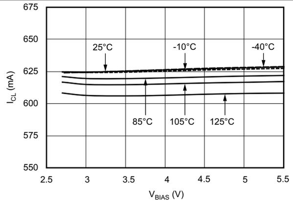
Figure 16. Current Limit vs  $V_{BIAS}$  Voltage
