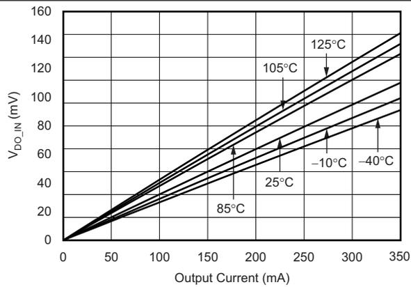
Figure 9.  $V_{IN}$  Dropout Voltage vs Output Current
