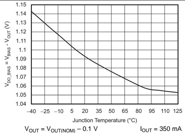
Figure 10.  $V_{BIAS}$  Dropout Voltage vs Junction Temperature
