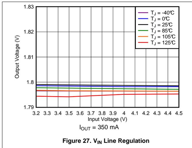
Figure 27.  $V_{IN}$  Line Regulation
