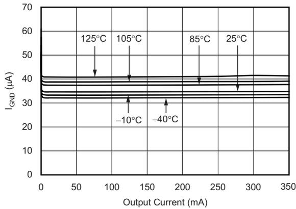
Figure 13. Ground Pin Current vs Output Current
