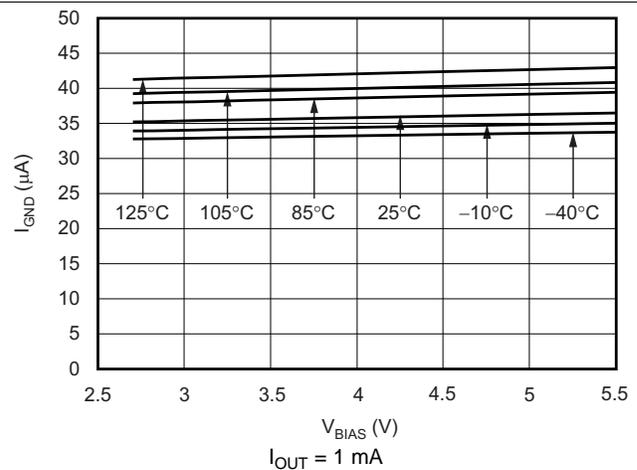
Figure 12. Ground Pin Current vs  $V_{BIAS}$  Voltage
