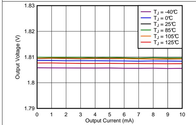
Figure 5. Load Regulation Under Light Loads
