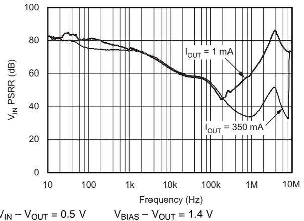
Figure 20.  $V_{BIAS}$  Power-Supply Rejection Ratio vs Frequency
