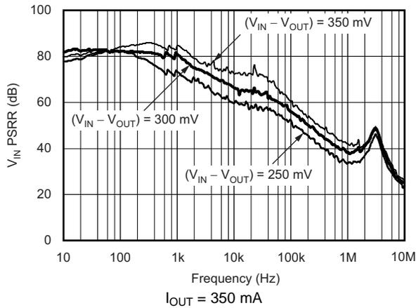
Figure 19.  $V_{IN}$  Power-Supply Rejection Ratio vs Frequency
