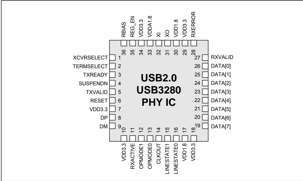
FIGURE 3-2: USB3280 PIN LAYOUT - BOTTOM VIEW
