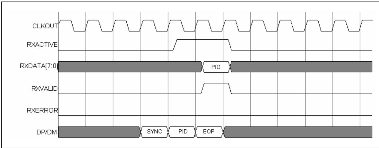
**FIGURE 7-6: RECEIVE TIMING FOR SETUP PACKET**
