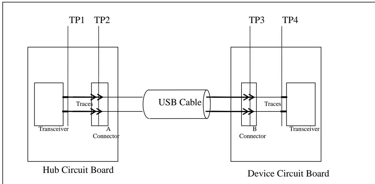
The eye pattern in Figure 6-4 defines the transmit waveform requirements for a hub (measured at TP2 of Figure 6-3) or a device without a captive cable (measured at TP3 of Figure 6-3). The corresponding signal levels and timings are given in table below. Time is specified as a percentage of the unit interval (UI), which represents the nominal bit duration for a 480 Mbit/s transmission rate.
