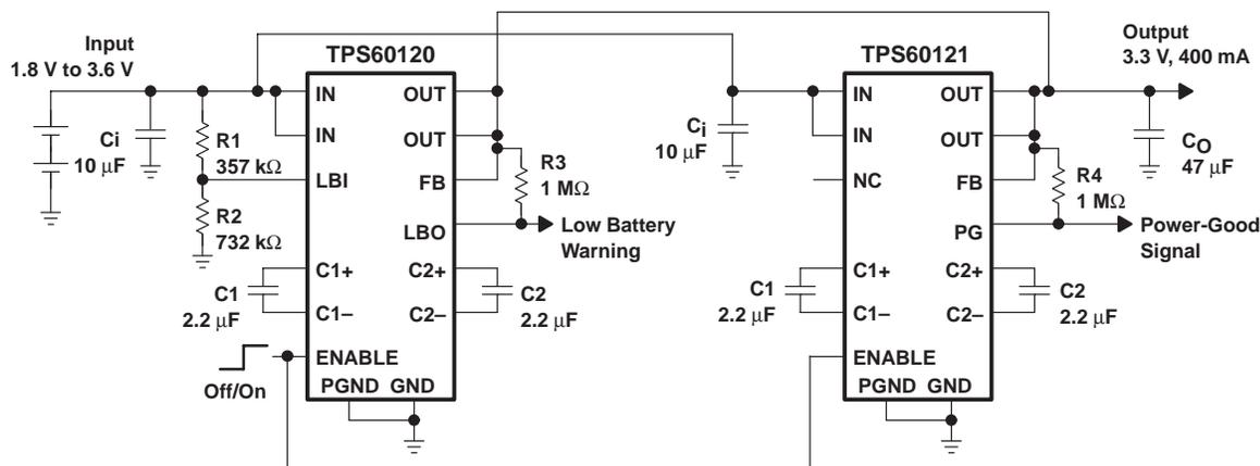
Figure 29. Paralleling of Two TPS6012x Charge Pumps
