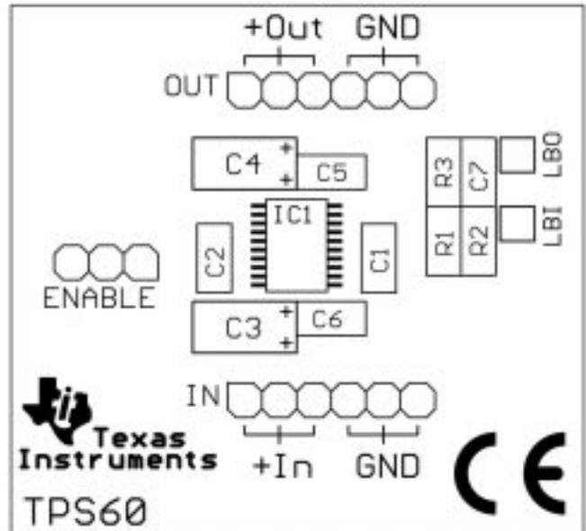
Figure 28. Component Placement
