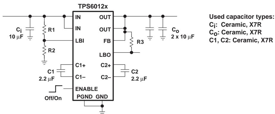
Figure 5. Circuit Used For Typical Characteristics Measurements
