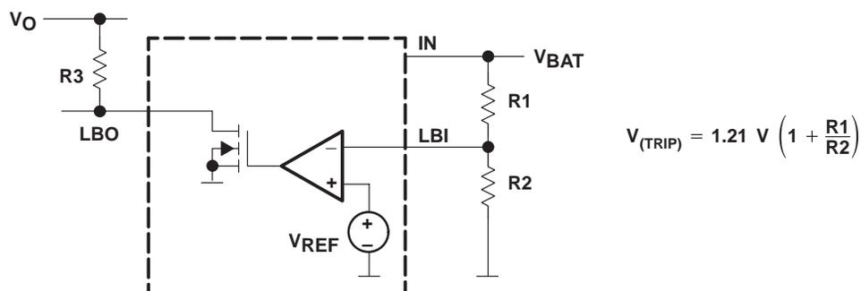
Figure 1. Programming of the Low-Battery Comparator Trip Voltage
