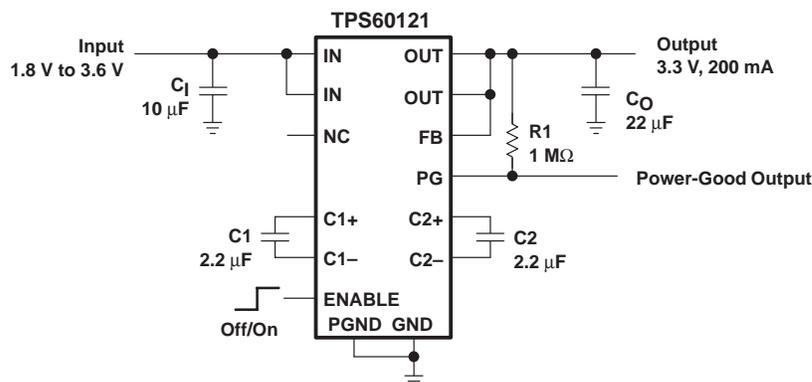
**Figure 2. Typical Operating Circuit Using Power-Good Comparator**
