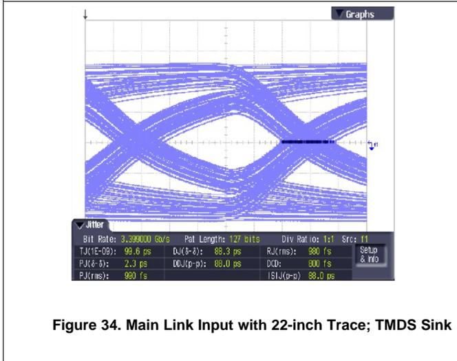
Figure 34. Main Link Input with 22-inch Trace; TMD5 Sink
