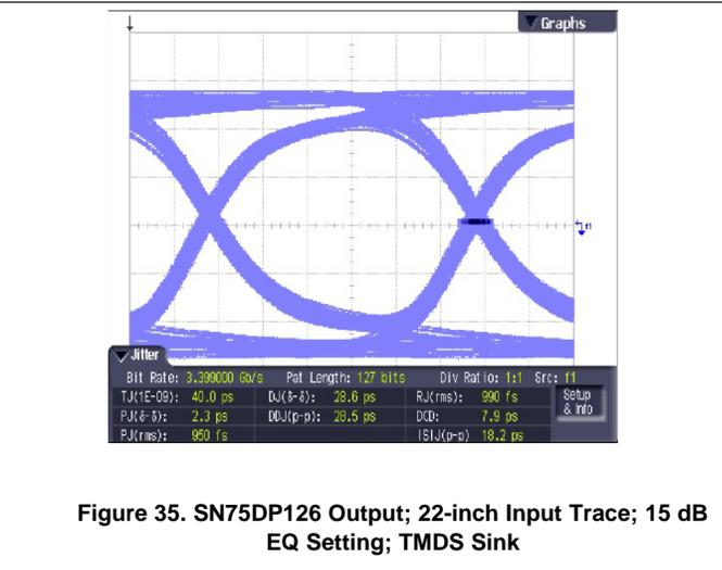
Figure 35. SN75DP126 Output; 22-inch Input Trace; 15 dB EQ Setting; TMD5 Sink
