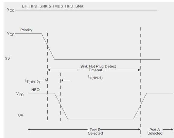
**Figure 8. HPD Timing Diagram #2**
