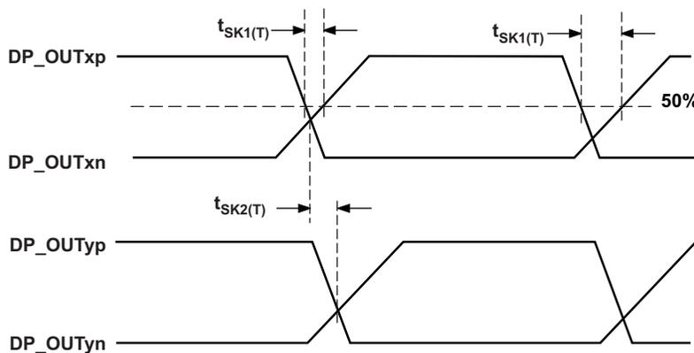
Figure 3. HDMI/DVI Sink TMD5 Output Skew Measurements
