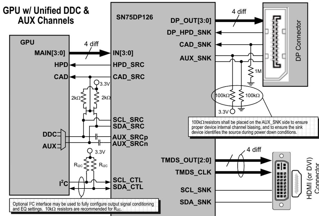
**Figure 24. GPU with a Unified AUX/DDC Configuration**
