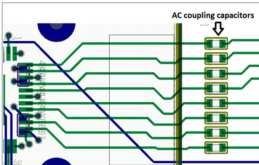
Figure 39. AC Capacitors Placement and Routing Example
