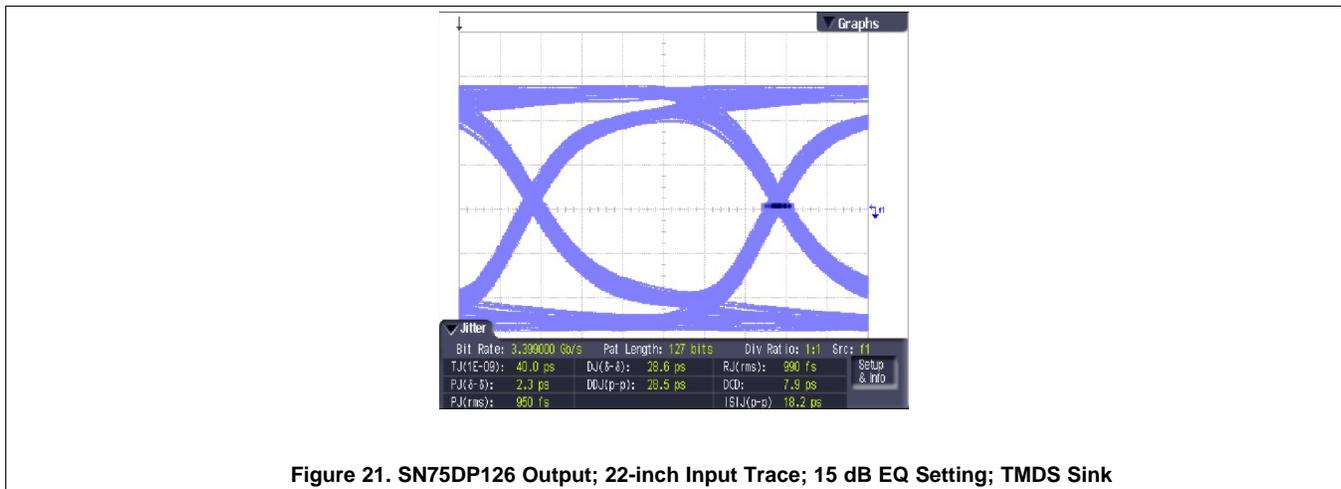
Figure 21. SN75DP126 Output; 22-inch Input Trace; 15 dB EQ Setting; TMD5 Sink
