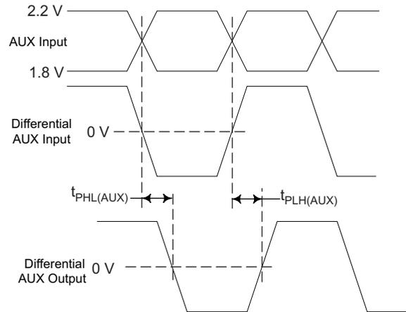
Figure 12. AUX Delay Measurement
