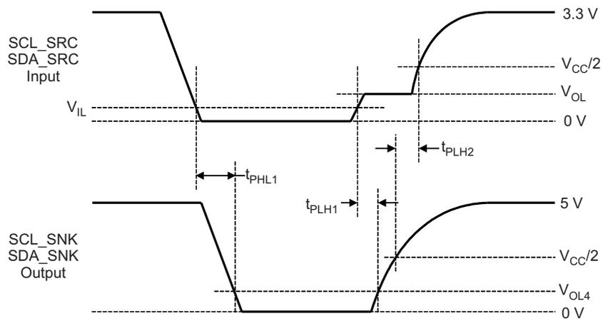
Figure 13. DDC Propagation Delay – Source to Sink
