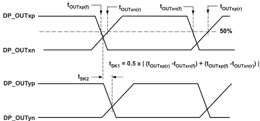
Figure 2. DisplayPort Sink Main Link Skew Measurements
