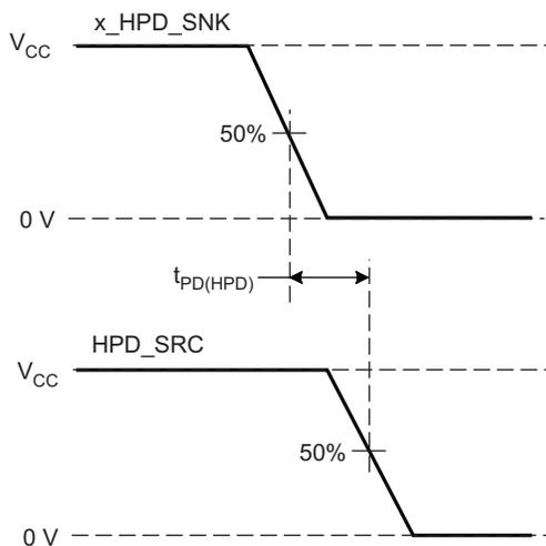
**Figure 7. HPD Timing Diagram #1**
