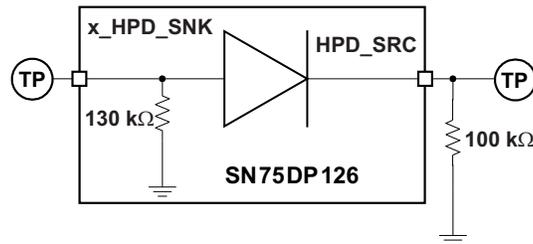
**Figure 6. HPD Test Circuit**
