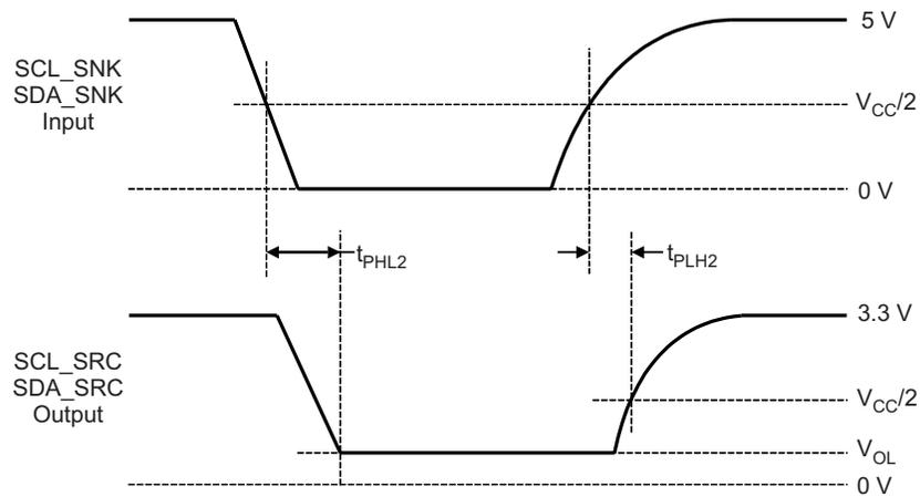
Figure 14. DDC Propagation Delay – Sink to Source
