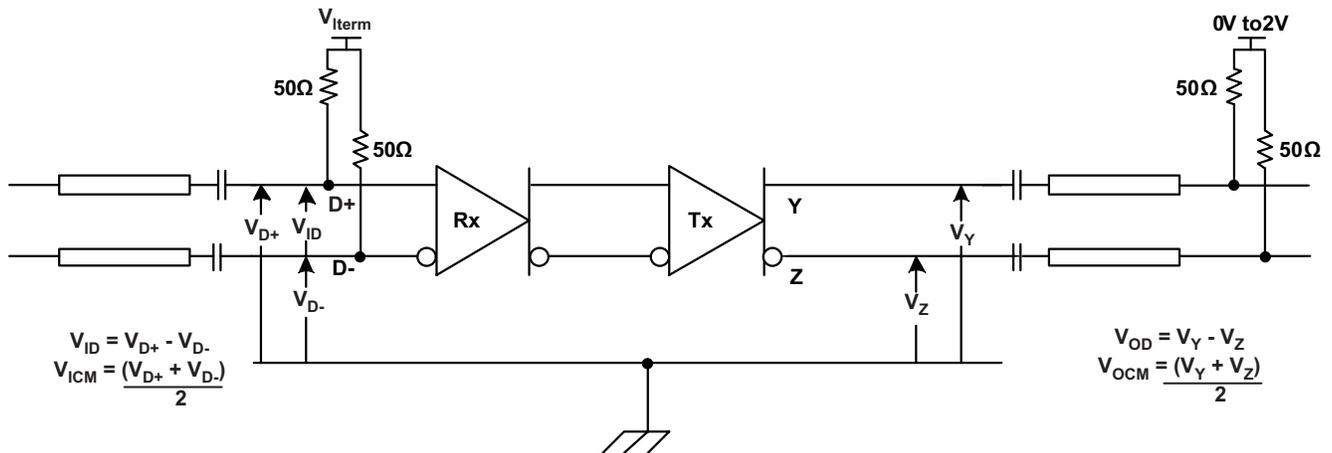
Figure 1. DisplayPort Sink Main Link Test Circuit
