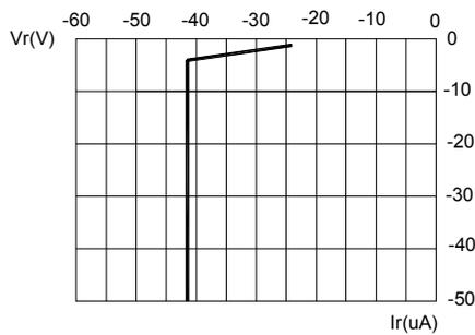
FIG.3 RED & AMBER REVERSE CURRENT VS. REVERSE VOLTAGE.
