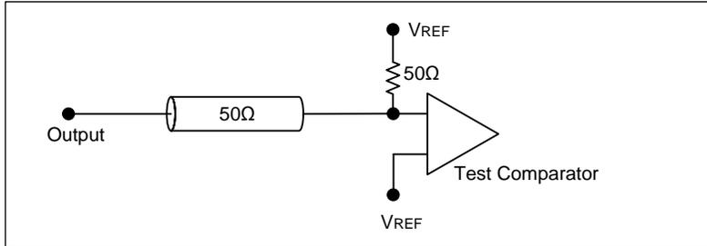
(b)  $t_{CHQZ}$  and  $t_{CHQX1}$  are specified with 5pF load capacitance and measured when transition occurs  $\pm 100\text{mV}$  from the steady state voltage.
