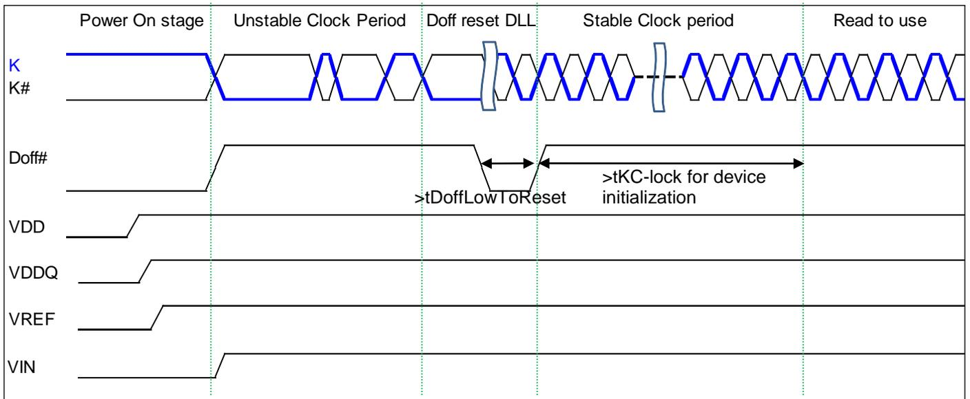
Note) Applying DLL reset sequences (sequence 3a, 3b) are also required when operating frequency is changed without power off.
