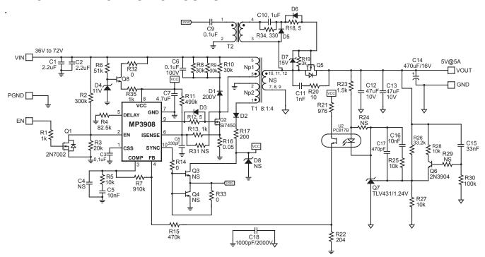
Figure 2—MP3908 Isolated Synchronous Flyback Application
