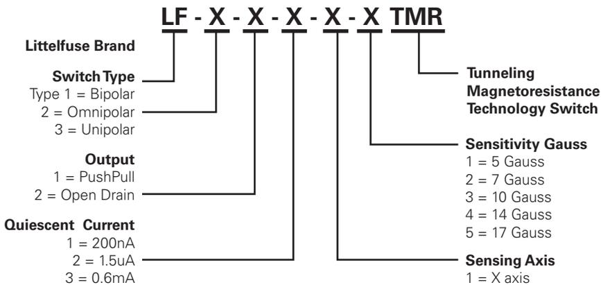
Example: LF32115TMR is an Omnipolar, PushPull, 1.5uA, X axis, 17 Gauss
