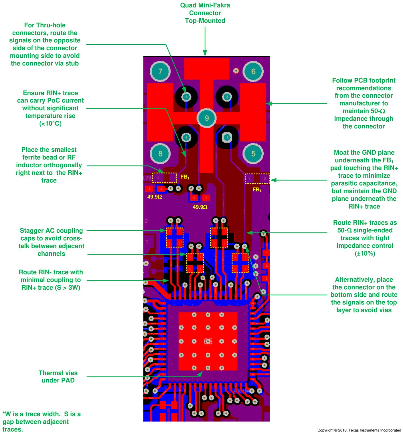
**Figure 10-1. DS90UB960-Q1 Example PCB Layout With Quad Mini-Fakra Connector**
