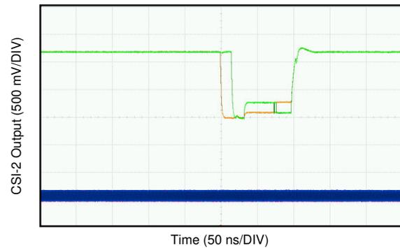
Figure 8-9. CSI-2 DATA and Continuous CLK Output
