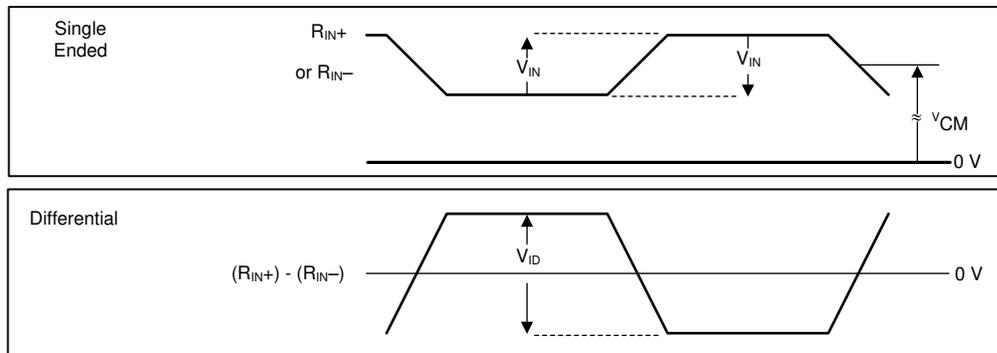
**Figure 6-2. FPD-Link Receiver VID, VIN , VCM**
