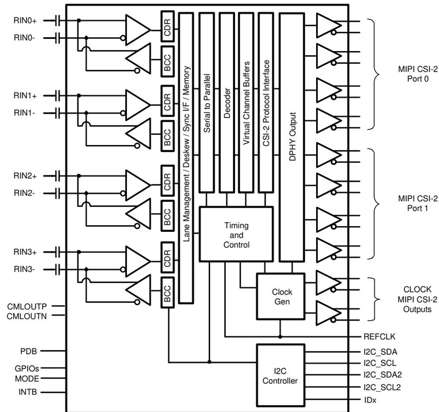
Figure 7-1. Functional Block Diagram
