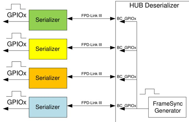
**Figure 7-17. Internal FrameSync**
