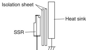
Please keep 5mm distance as minimum between naked metal portion of SSR and heat sink, and also between naked metal portion of SSR and bis/nut/washer. However, please avoid the natural rubber for isolation sheet.
