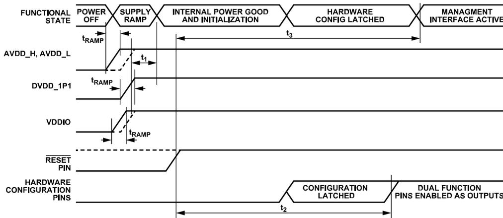
Figure 2. Power-Up Timing
