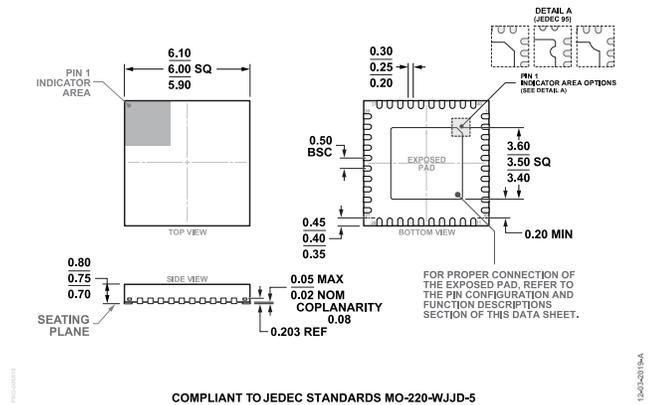
**Figure 26. 40-Lead Lead Frame Chip Scale Package [LFCSP]
