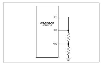
Figure 3. Resistive Divider from REF
