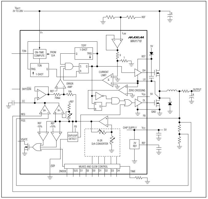
Figure 2. Functional Diagram
