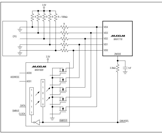
Figure 14. Using the ZMODE Multiplexer
