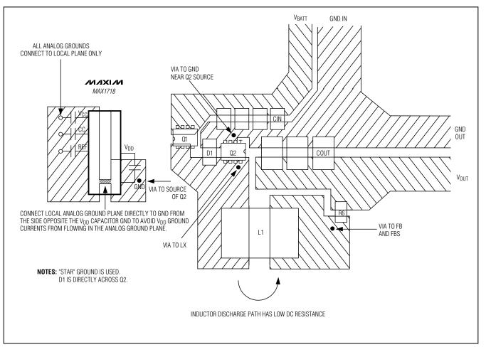
Figure 19. Power-Stage PC Board Layout Example
