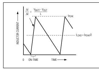
Figure 6. Pulse-Skipping/Discontinuous Crossover Point
