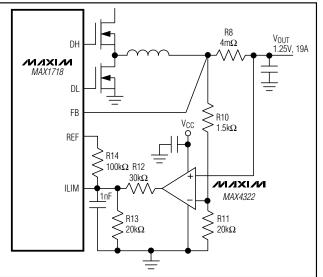
Figure 16. Improving Current-Limit Accuracy
