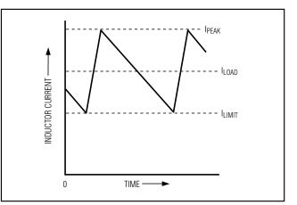
Figure 7. "Valley" Current-Limit Threshold Point
