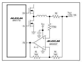
Figure 15. Lowering Voltage-Positioning Power Dissipation
