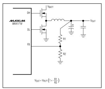
Figure 18. Adjusting VOUT with a Resistor-Divider
