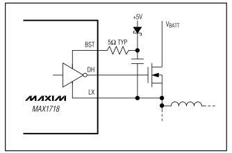
Figure 8. Reducing the Switching-Node Rise Time
