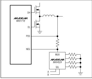
Figure 5. Programmable Offset Voltage
