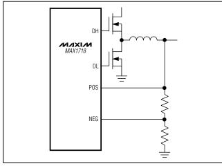
Figure 4. Resistive Divider from OUTPUT
