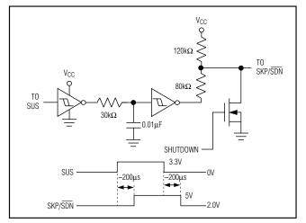
Figure 17. Using Skip Mode During Suspend (SKP/ $\overline{SDN} = V_{CC}$ )
