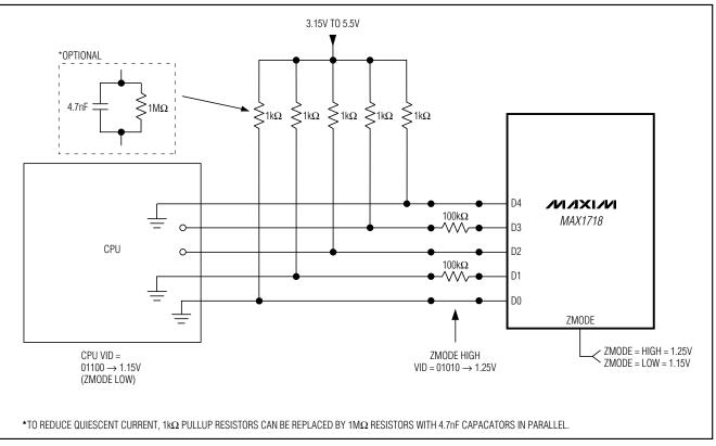
Figure 13. Using the Internal Mux with CPU Driving the Logic-Mode VID Code
