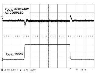
FIGURE 8. LOAD TRANSIENT RESPONSE VOUT2 (3.3V)
