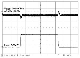
FIGURE 7. LOAD TRANSIENT RESPONSE VOUT1 (3.3V)
