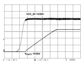
FIGURE 9. PWM SOFT-START WAVEFORM
