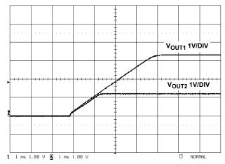
FIGURE 14. PWM1 AND PWM2 OUTPUT TRACKING DURING STARTUP
