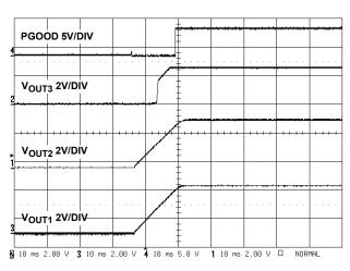
FIGURE 4. SOFT-START WAVEFORMS WITH PGOOD
