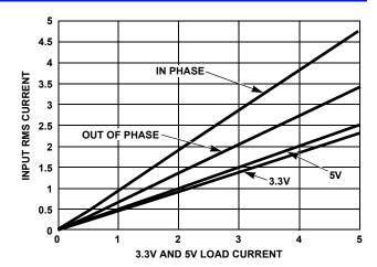
FIGURE 20. INPUT RMS CURRENT vs LOAD
