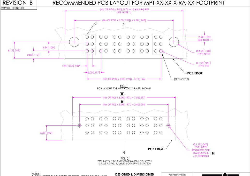
CONNECTOR ENVELOPE DIMENSIONS. OTHER COMPONENTS PLACED ON PCB SHALL AVOID THIS ZONE.
