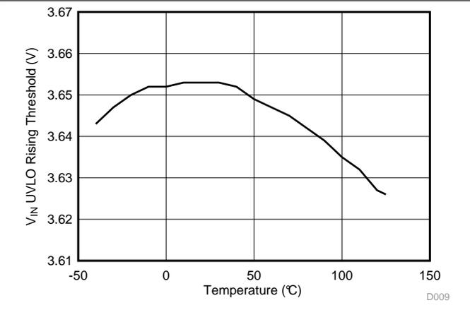
Figure 10.  $V_{IN}$  UVLO Rising Threshold vs Junction Temperature
