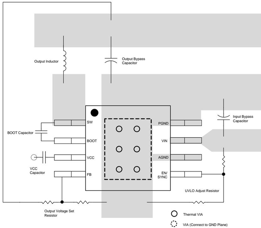
**Figure 34. SOIC Layout**
