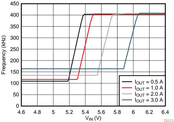
Figure 20. Frequency Foldback at Dropout (V<sub>OUT</sub> = 5 V, f<sub>SW</sub> = 400 kHz)
