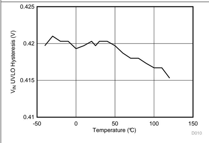
Figure 11.  $V_{IN}$  UVLO Hysteresis vs Junction Temperature
