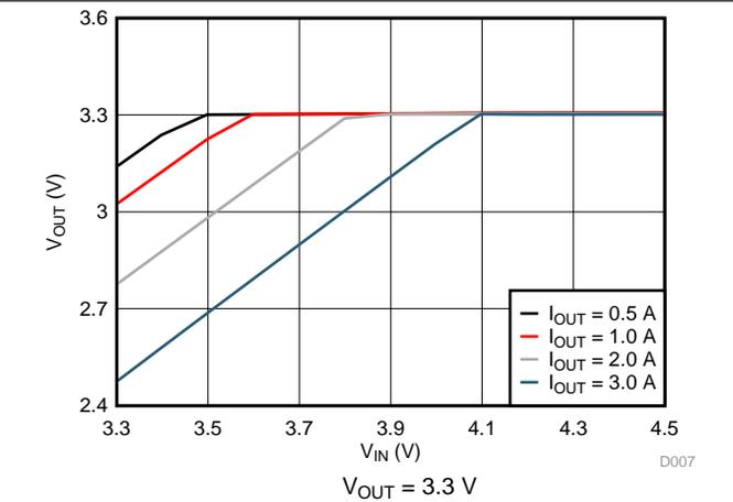
Figure 8. Dropout Curve
