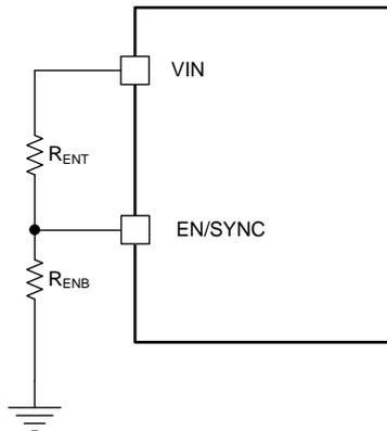
Figure 16. System UVLO by Enable Divider
