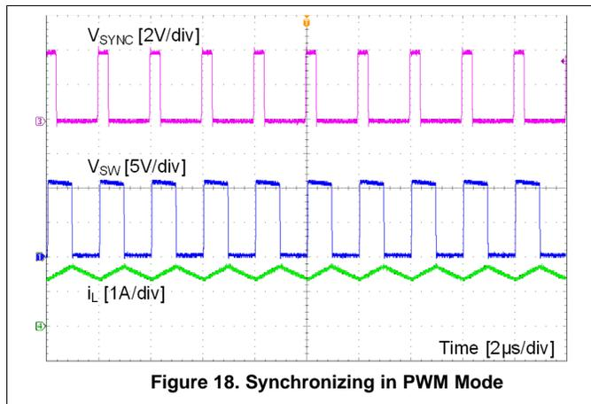
Figure 18. Synchronizing in PWM Mode
