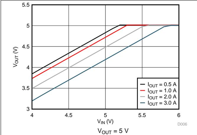
Figure 7. Dropout Curve
