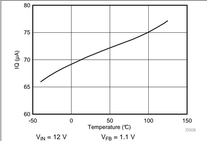
Figure 9.  $I_Q$  vs Junction Temperature
