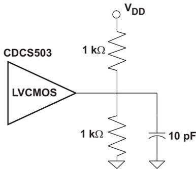
**Figure 2. Test Load**
