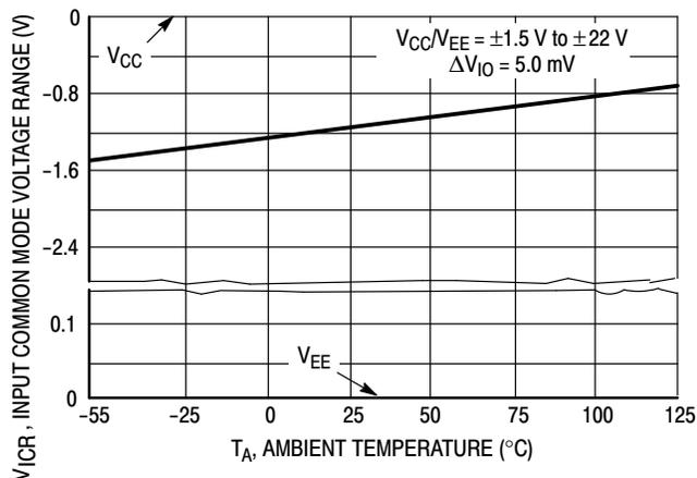
**Figure 2. Input Common Mode Voltage Range versus Temperature**
