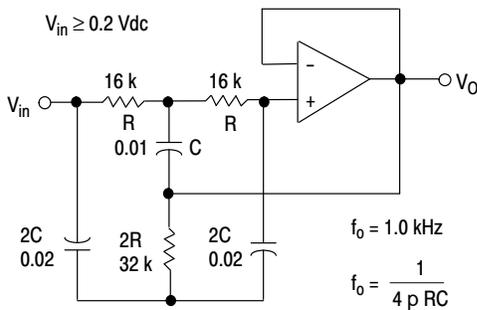
**Figure 14. Active High-Q Notch Filter**
