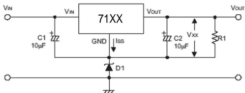
$$V_{OUT} = V_{xx} + VD1$$
