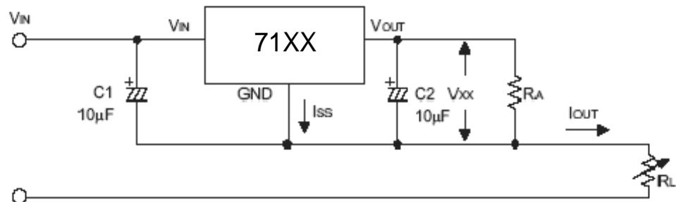
$$I_{OUT} = V_{xx}/R_A + I_{SS}$$
