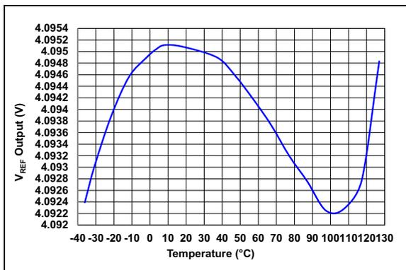
**FIGURE 3-3:** MCP1502-40  $V_{REF}$  Output vs. Temperature,  $V_{DD} = 5.5V$ .
