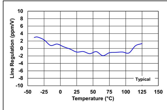
**FIGURE 3-6:** MCP1502 – Line Regulation vs. Temperature.
