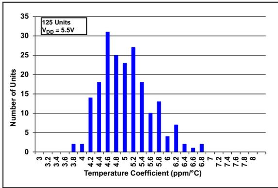
**FIGURE 3-13:** MCP1502 Tempco Distribution, No Load,  $V_{DD} = 5.5V$ .
