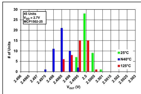
**FIGURE 3-18:** MCP1502 Output Voltage Histogram,  $V_{DD} = 2.7V$ .
