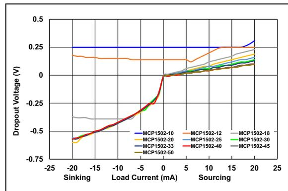
**FIGURE 3-11:** Dropout Voltage vs. Load,  $T_A = +25^\circ C$ .
