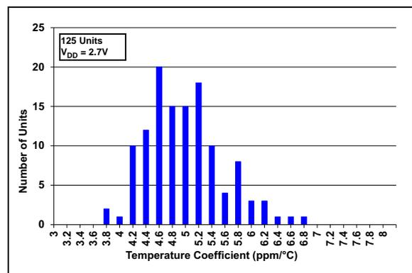
**FIGURE 3-12:** MCP1502 Tempco Distribution, No Load,  $V_{DD} = 2.7V$ .
