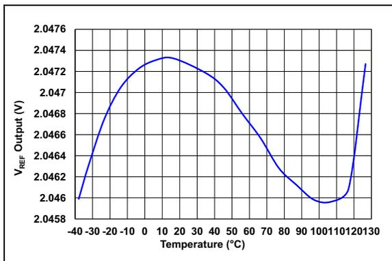
**FIGURE 3-2:** MCP1502-20  $V_{REF}$  Output vs. Temperature,  $V_{DD} = 5.5V$ .
