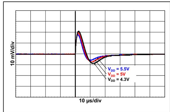
**FIGURE 3-34:** MCP1502-40 Transient Response vs.  $V_{DD}$ ,  $C_L = 4.7 nF$ .
