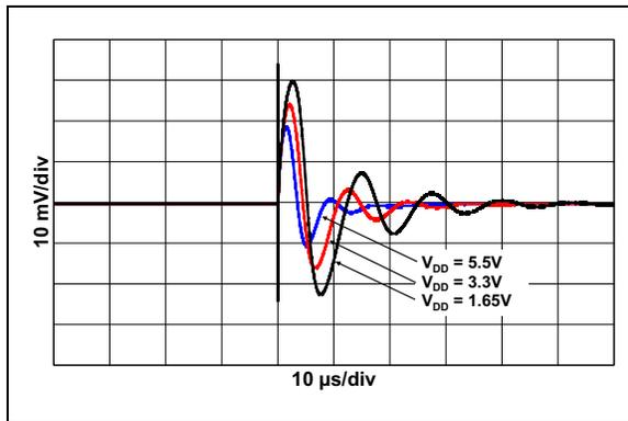
**FIGURE 3-32:** MCP1502-10 Transient Response vs.  $V_{DD}$ ,  $C_L = 4.7 nF$ .
