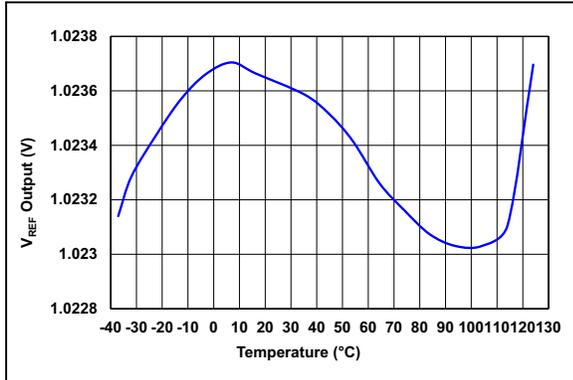
**FIGURE 3-1:** MCP1502-10  $V_{REF}$  Output vs. Temperature,  $V_{DD} = 5.5V$ .
