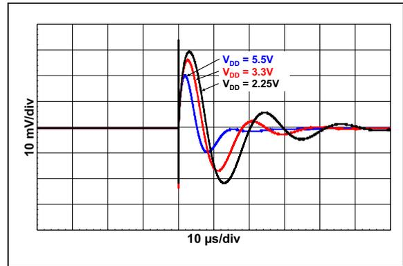
**FIGURE 3-33:** MCP1502-20 Transient Response vs.  $V_{DD}$ ,  $C_L = 4.7 nF$ .
