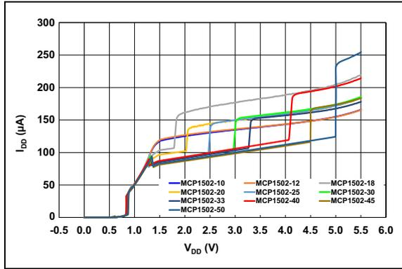
**FIGURE 3-7:**  $I_{DD}$  vs.  $V_{DD}$  for All Options.
