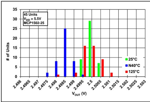
**FIGURE 3-19:** MCP1502 Output Voltage Histogram,  $V_{DD} = 5.5V$ .
