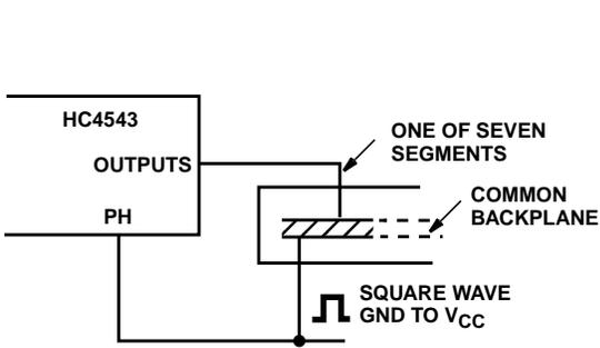
FIGURE 5. CONNECTION TO LIQUID-CRYSTAL (LCD) DISPLAY READOUT
