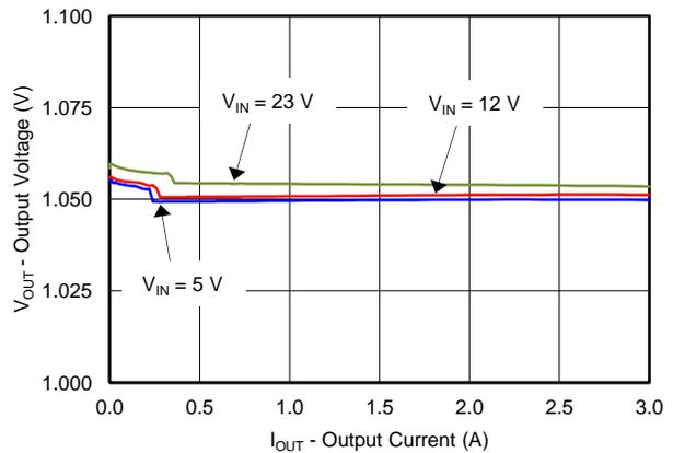
Figure 4. 1.05-V OUTPUT VOLTAGE vs OUTPUT CURRENT
