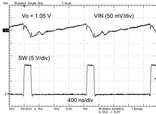
Figure 15. VOLTAGE RIPPLE AT INPUT (Io = 3 A)
