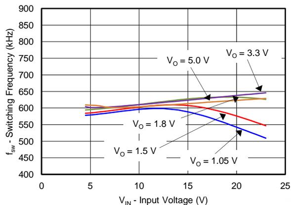
Figure 10. SWITCHING FREQUENCY vs INPUT VOLTAGE (I<sub>O</sub> = 1 A)
