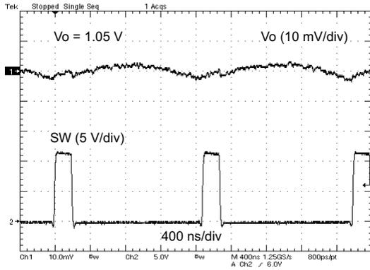
Figure 13. VOLTAGE RIPPLE AT OUTPUT (Io = 3A)
