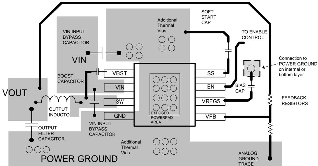
Figure 18. PCB Layout
