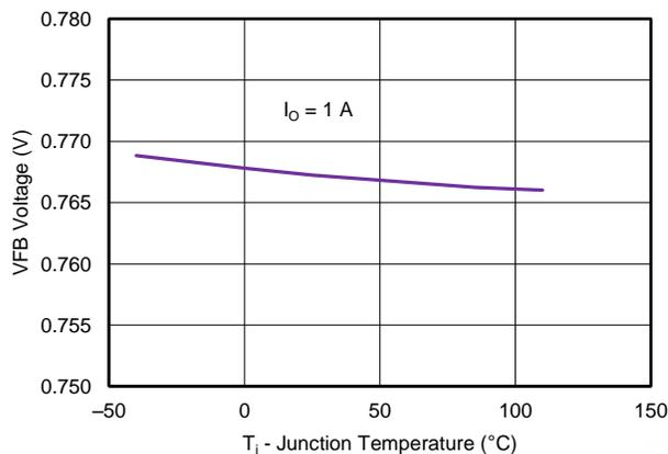
Figure 12. VFB VOLTAGE vs JUNCTION TEMPERATURE (I<sub>O</sub> = 1 A)
