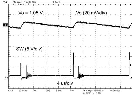
Figure 14. VOLTAGE RIPPLE AT OUTPUT (Io = 30 mA)
