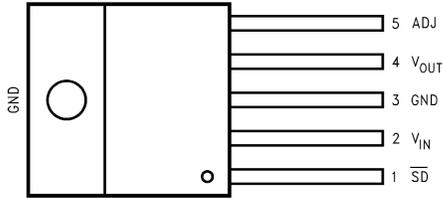
Figure 1. TO-220-5 Package (Top View) Bent, Staggered Leads
