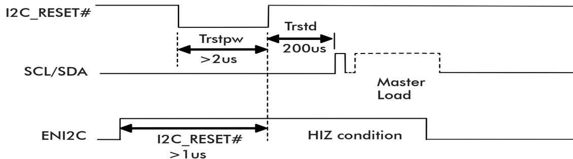
**Figure 5-1 I2C Reset, Enable and SCL/SDA Timing Diagram**
