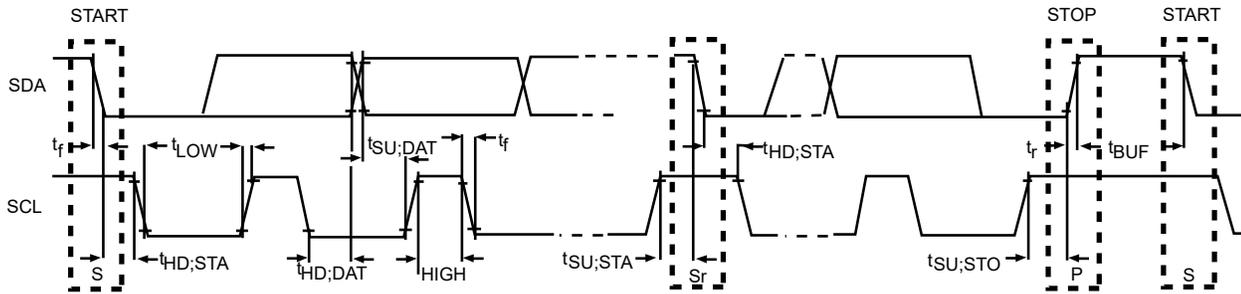
Figure 6-7 I<sup>2</sup>C Timing Diagram
