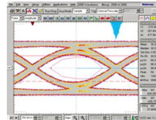
**Figure 7-7 Output Eye Diagram at FG 0.5dB**
