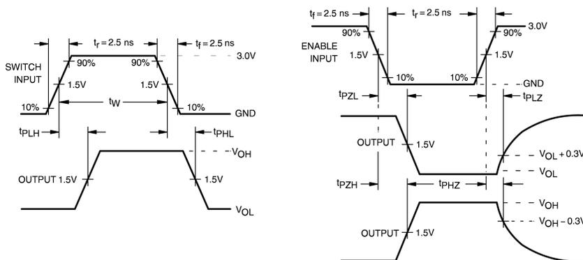
FIGURE 2. AC Waveforms
