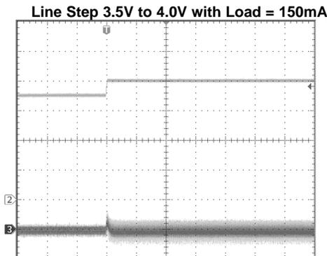
CH2:  $V_{IN}$ ; Scale: 1V/Div, DC Coupled
