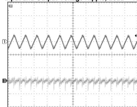
CH1:  $V_{IN}$ , Scale: 50mV/Div, AC Coupled
