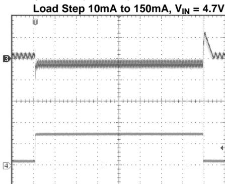
CH3:  $V_{OUT}$ ; Scale: 50mV/Div, AC Coupled
