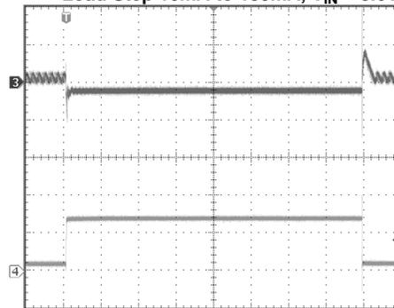
CH3:  $V_{OUT}$ , Scale: 50mV/Div, AC Coupled
