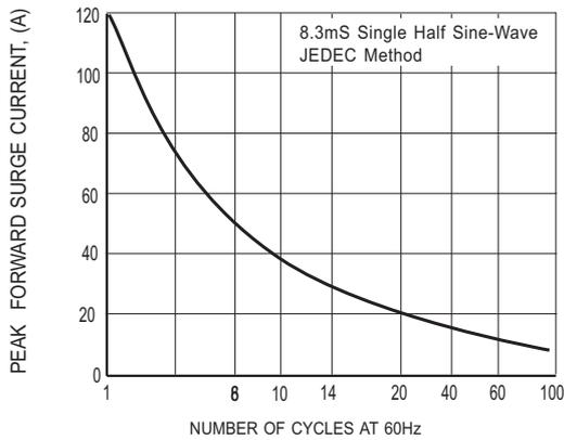
FIG. 1 - TYPICAL NON-REPETITIVE FORWARD SURGE CURRENT
