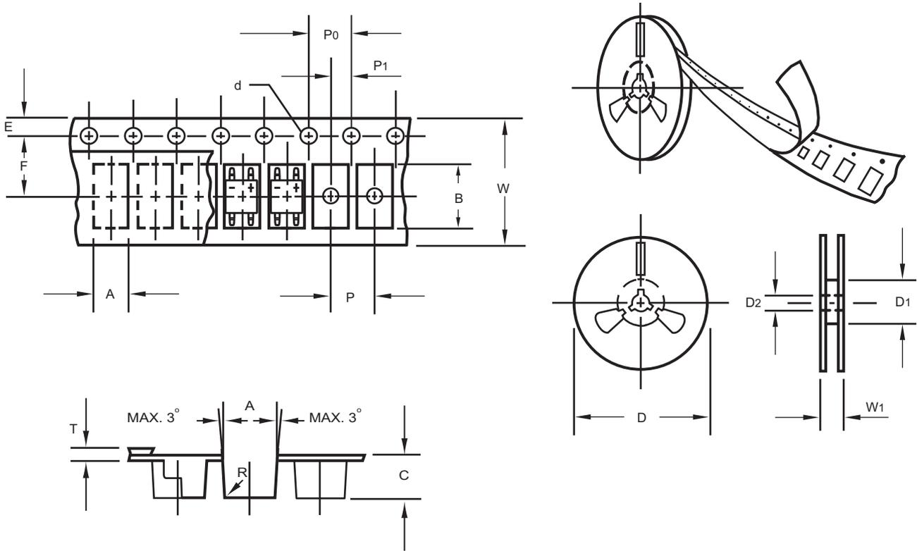
Fig.: Configuration of SLDBS TAPING
