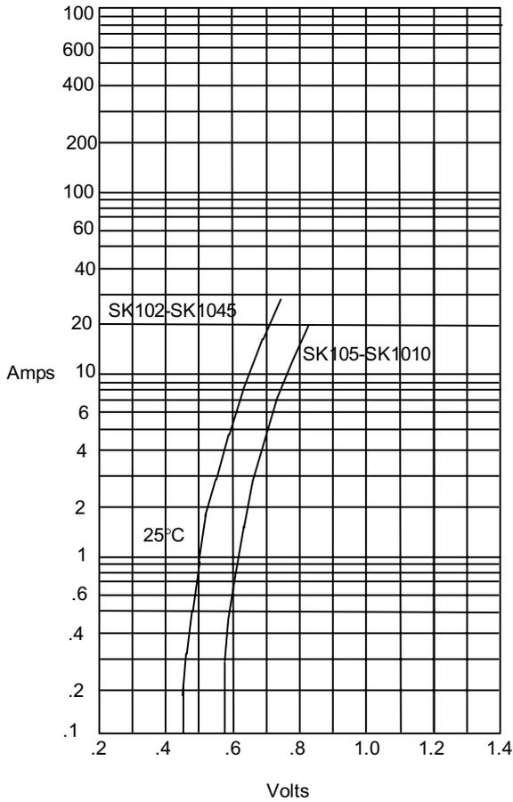
Instantaneous Forward Current - Amperes *versus*
