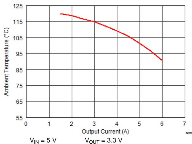
Figure 38. Maximum Ambient Temperature for  $T_J=125^\circ\text{C}$  (TPSM82480 EVM)
