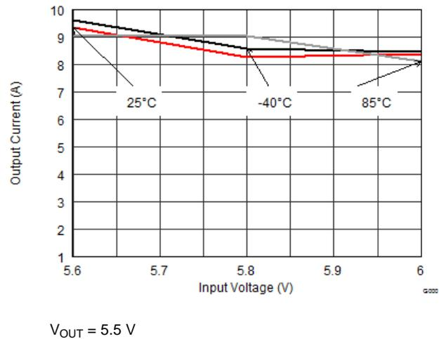
Figure 19. Maximum Output Current
