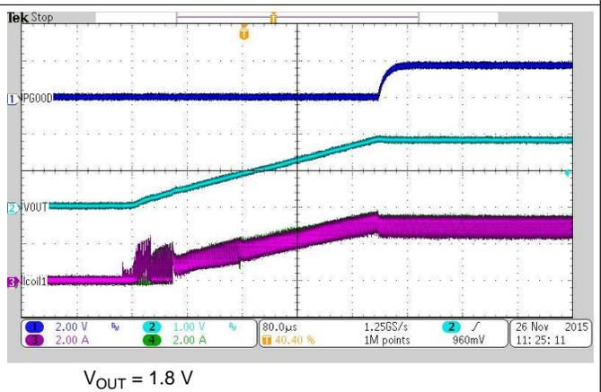
Figure 25. Startup into 0.3  $\Omega$  resistor
