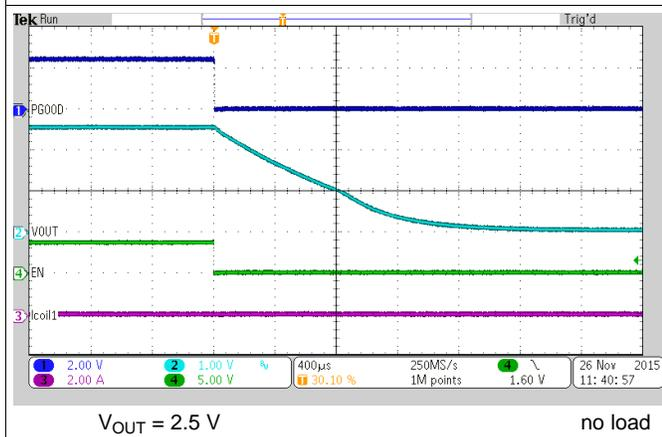
Figure 26. Output Discharge
