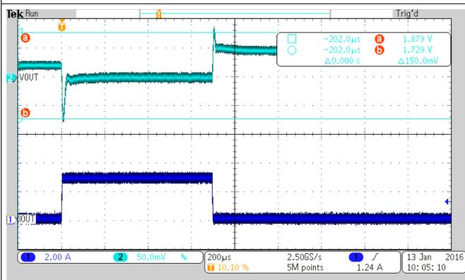
Figure 32. Load Transient Response (PSM-PWM), Load Step 0 to 3 A
