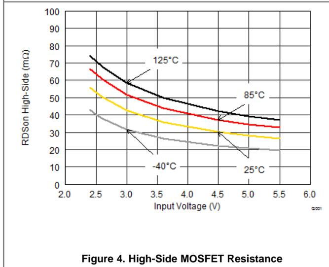
**Figure 4. High-Side MOSFET Resistance**
