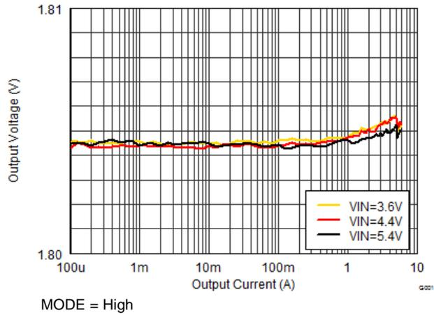
Figure 16. Output Voltage vs Output Current (Load Regulation)
