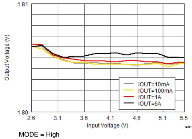
Figure 17. Output Voltage vs Input Voltage (Line Regulation)
