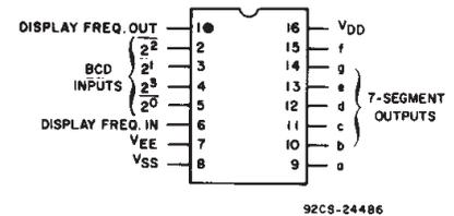
transferred from input to output by placing a high voltage level at the strobe input. A low voltage level at the strobe input latches the data input and the corresponding output segments remain selected (or non-selected) while the strobe is low.
