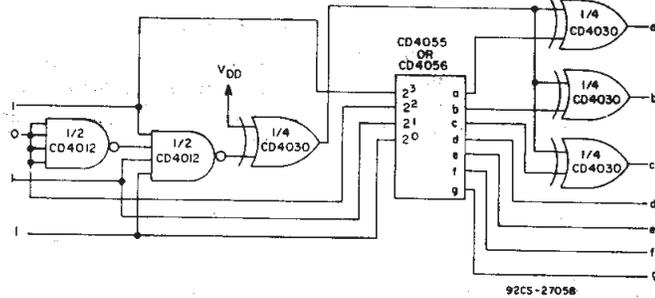
Fig. 21 - Conversion of "H" display to "F" display.
