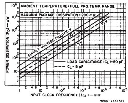
Fig. 7 - Typical input clock frequency vs. power dissipation.
