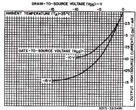
Fig. 10 - Typical p-channel output high (source) current characteristics.
