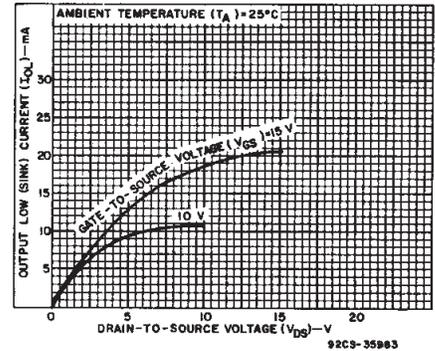
Fig. 8 - Typical n-channel output low (sink) current characteristics.
