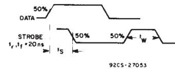
Fig. 15 - Data setup time and strobe pulse duration.
