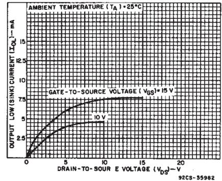
Fig. 9 - Minimum n-channel output low (sink) current characteristics.
