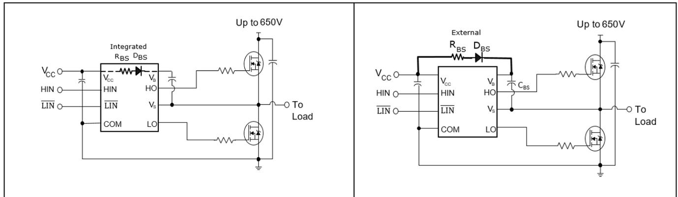
**Figure 12** 2ED210x with integrated components **Figure 13** Standard bootstrap gate driver
