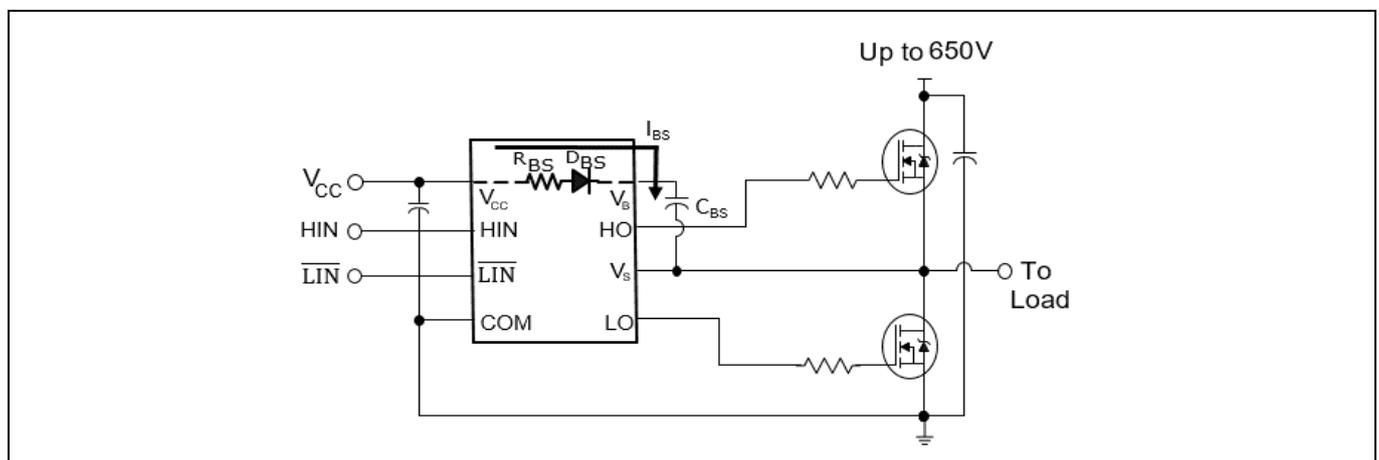
**Figure 14** Half bridge bootstrap circuit in 2ED210x
