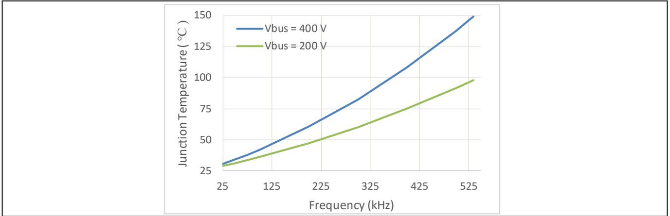
\* Assumptions for above curves: LLC topology, Power switch = IPP60R600P6,  $T_a = 25\text{ }^\circ\text{C}$ ,  $V_{BUS} = 400\text{ V}$ ,  $V_{CC} = 12\text{ V}$ ,  $R_{gon} = 15\text{ }\Omega$ ,  $R_{goff} = 12\text{ }\Omega$
