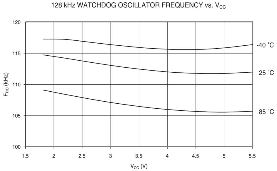
**Figure 19-57.** 128 kHz Watchdog Oscillator Frequency vs. Temperature
