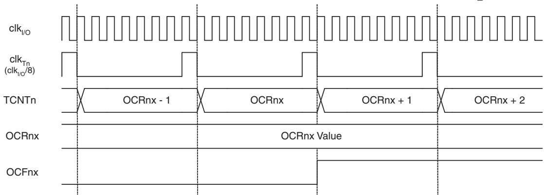
Figure 11-11 on page 69 shows the setting of OCF0A and the clearing of TCNT0 in CTC mode and fast PWM mode where OCR0A is TOP.
