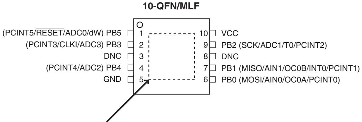
NOTE: Bottom pad should be soldered to ground.
