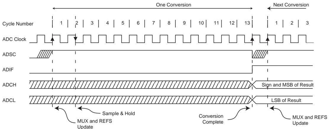
When Auto Triggering is used, the prescaler is reset when the trigger event occurs, as shown in [Figure 14-6](#) below. This assures a fixed delay from the trigger event to the start of conversion. In this mode, the sample-and-hold takes place two ADC clock cycles after the rising edge on the trigger source signal. Three additional CPU clock cycles are used for synchronization logic. Three additional CPU clock cycles are used for synchronization logic.
