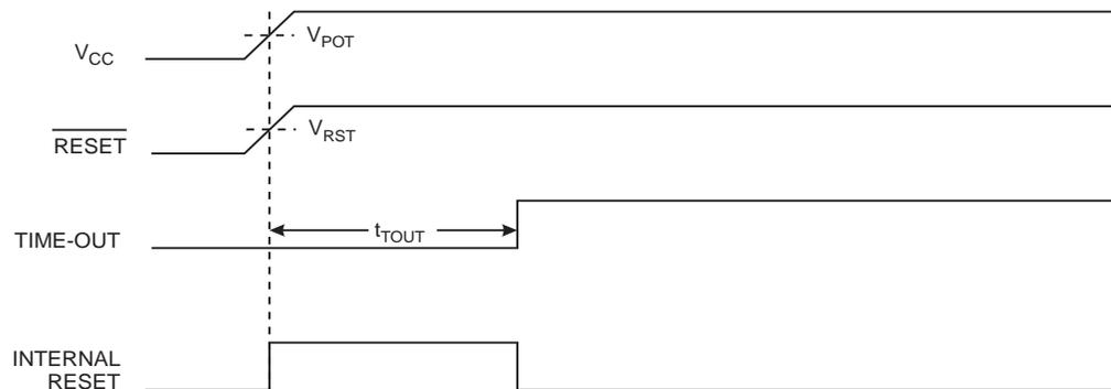
**Figure 8-3.** MCU Start-up,  $\overline{RESET}$  Extended Externally
