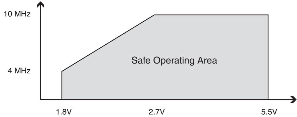
**Figure 18-2.** Maximum Frequency vs.  $V_{CC}$  for ATTiny13
