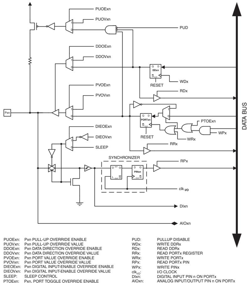
Note: WRx, WPx, WDx, RRx, RPx, and RDx are common to all pins within the same port.  $clk_{I/O}$ , SLEEP, and PUD are common to all ports. All other signals are unique for each pin.
