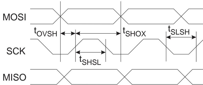
Figure 18-5. Serial Programming Waveform
