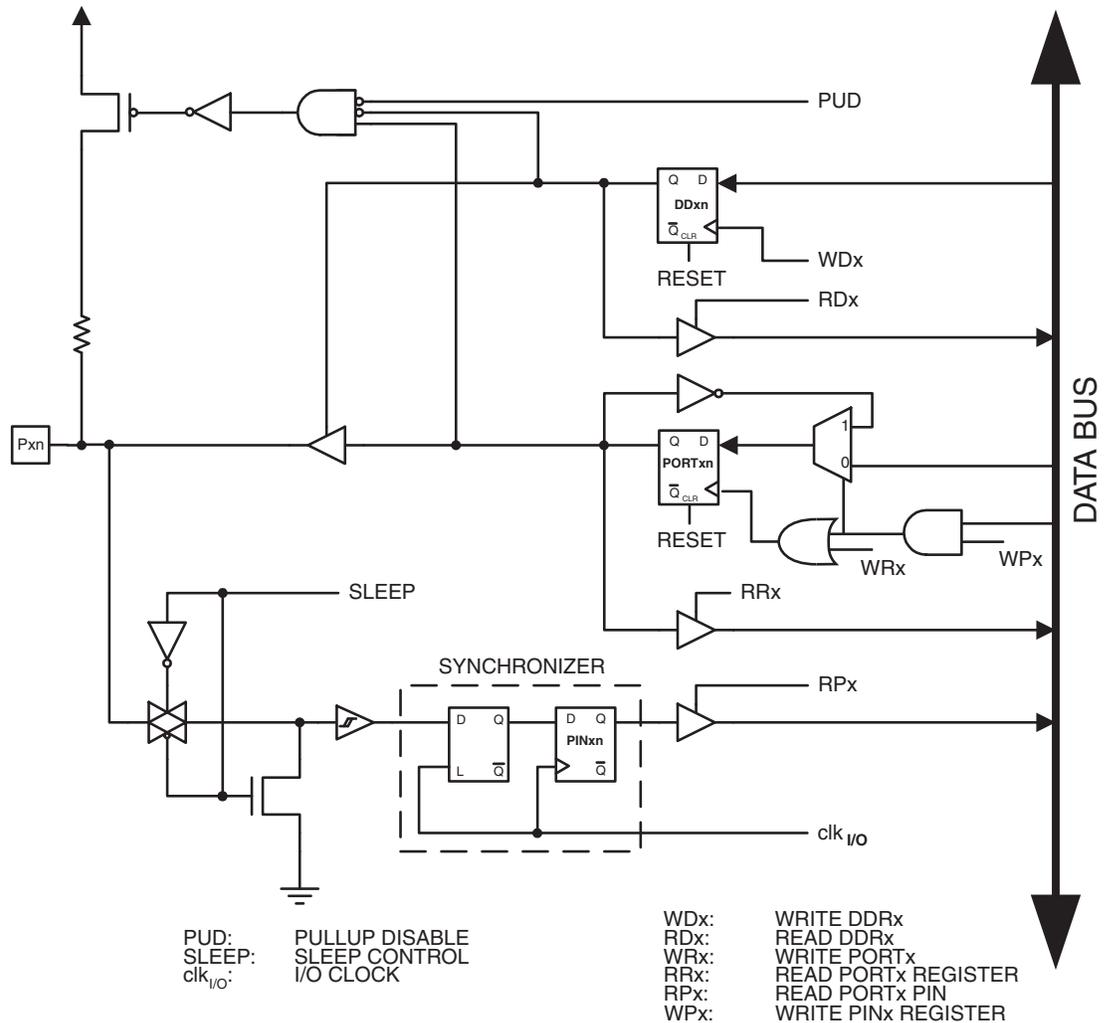
Note: 1. WRx, WPx, WDx, RRx, RPx, and RDx are common to all pins within the same port. clk<sub>I/O</sub>, SLEEP, and PUD are common to all ports.
