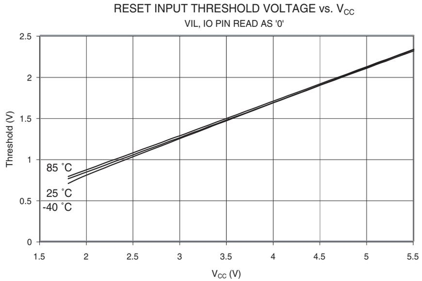
**Figure 19-45.** Reset Input Pin Hysteresis vs.  $V_{CC}$
