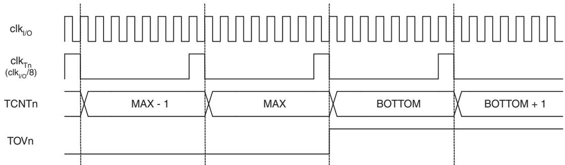
Figure 11-10 shows the setting of OCF0B in all modes and OCF0A in all modes except CTC mode and PWM mode, where OCR0A is TOP.
