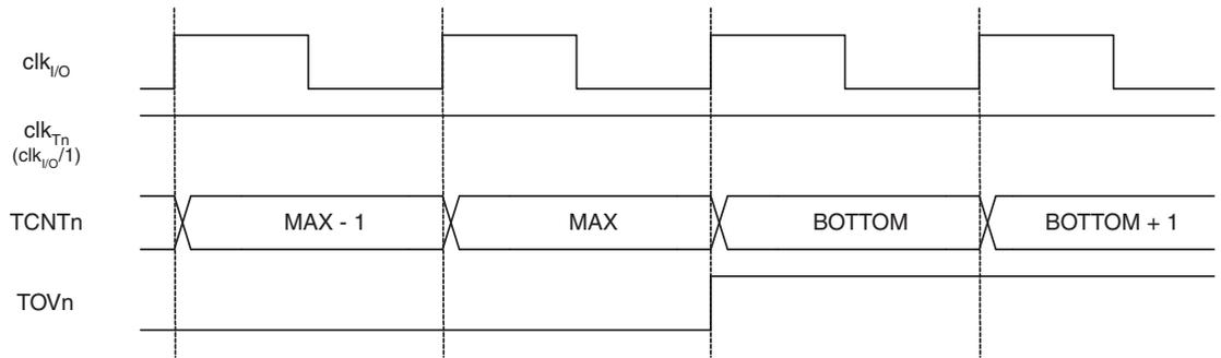
Figure 11-9 shows the same timing data, but with the prescaler enabled.
