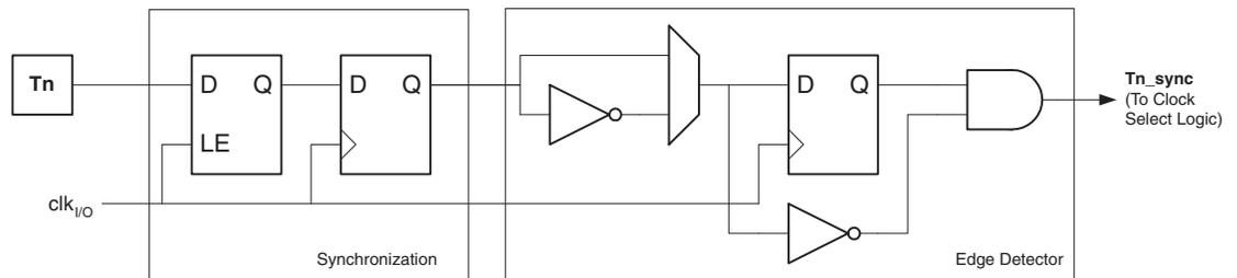
The synchronization and edge detector logic introduces a delay of 2.5 to 3.5 system clock cycles from an edge has been applied to the T0 pin to the counter is updated.
