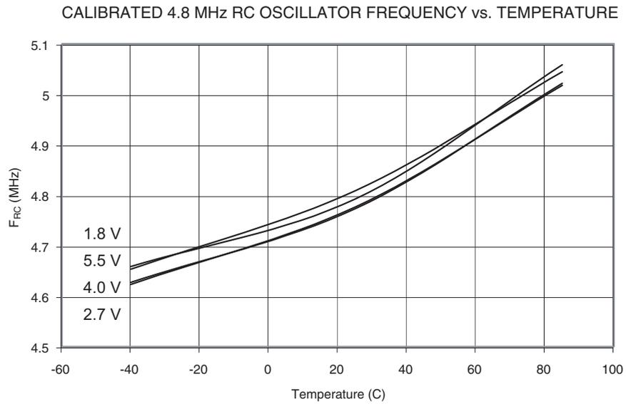
**Figure 19-54.** Calibrated 4.8 MHz RC Oscillator Frequency vs.  $V_{CC}$
