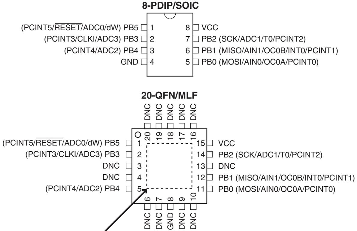
NOTE: Bottom pad should be soldered to ground.
